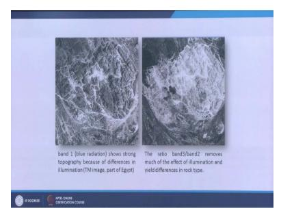
Now, we see the output, here a blue radiation means band 1 and since the strong topography while the strong topography is visible, because of differences in illumination, it's a hilly terrain, rugged terrain and when illumination is there, there will be some shadow in the hilly terrain and that will show the depth perception as well, so if we want to deemphasize the depth perception, then we need to involve some band rationing.
