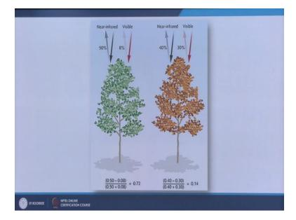
How this works is very simple as I explained that in near infrared and the healthy vegetation will say roughly reflect in this particular example about 50 percent radiation, whereas in visible part
