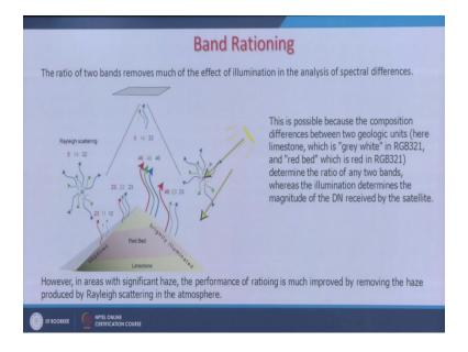
Now, in the band receiving, the ratio of two bands removed, much of the effects of illumination in the analysis of spectral differences. If you are having too much shadow areas and bright areas and shadow areas, you involve two bands and create a ratio, you would find that the shadow effect have reduced and this is what it is... that solar illumination is here, we don't bother much about the scattering which is happening in this atmosphere.
