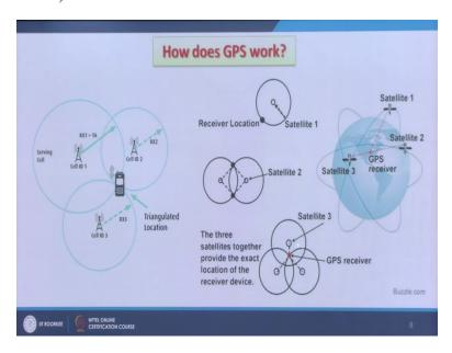
So we will be we will we will go on further on this how GPS works basically as I have been saying that this the this like in case of towers, mobile towers, how they get the concept of a GPS, how they get the signal, that each tower, if each tower keeps transmitting its location as well apart from signals then wherever these 3 (sig) you know the range of these towers that means these circles, 3 circles will cut that is the position where I am standing.
