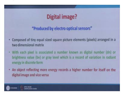
Digital image basically produce by electro optical sensors, so these sensors whether it is a on a satellite or any other devices they are all so there is lot of similarity between these table top or flatbed scanners and the scanners which are in space they scan line by line they produce, they produce images of any document or map of part of the earth using this concept of electro optical sensors.
