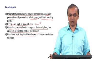
So to conclude our discussion on the magnetohydrodynamic power generation process so, the magnetohydrodynamic power generation process, enables us to generate power from hot gases without moving parts. So, I think that's something that we have to emphasize here, normally we are looking at you know in any thermal power plant and so on, you are looking at some moving part.
