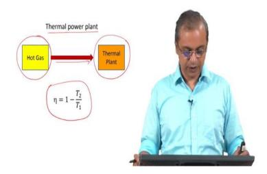
So, as I suggest said you know in a typical thermal power plant that's our scheme of operation. So, we have some hot gas that is coming in, and that's essentially sent towards the thermal plant, and in the thermal plant we are generating electricity. So, that is the general scheme of operation that we have, and as I just mentioned this is our efficiency limit ok. So, that is basically what we are trying to do.
