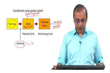
So, this is where we create this we utilize this magneto hydrodynamic generation process ok. So, this MHD process is utilized in this context it's the magnetohydrodynamic energy generation process is used, in this context of utilizing the process flow that's already happening in a thermal plant, and sort of introducing this into that process flow to see if you can extract some more energy out of that fuel.
