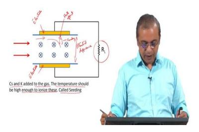
So, this is the basic idea. So, you get voltage potential difference, now you will get a potential difference here, and so you put an electrode here this is an electrode, and this is another electrode or a current collector ok. So, you put 2 electrodes, and you generate a you it's the system is already generated a potential the potential difference.
