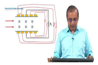
So I have a series of electrodes on top, I have a series of electrodes in the bottom, and I can pick them up in pairs. So, for example, I have shown you 1 path that I have picked up 1 pair here right. So, I picked up 1 pair here which is then connected to this load resistor. Similarly I can pick other pair. So, for example, I can pick this pair then I can
