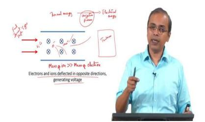
So let me put it here, mass of ion is much much greater than mass of electron, right mass of ion is much much greater than the mass of the electron. So, therefore, given the same amount of magnetic field, and the fact that it is all coming in the plasma to together, the extent to which the ion will deflect it will be lot less than the extent to which the electron will deflect.
