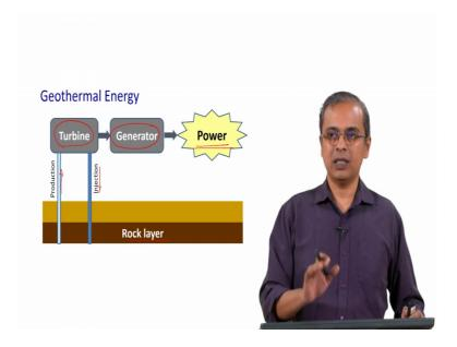
Geothermal energy, this is energy that is already there inside the earth. So, if you go deep inside the earth maybe even you know say one and half, 1- 2; say to 1, 2 or 3 kilo meters deep into the earth you see temperatures that are extremely hot right. And in fact the I mean some representation of this is what we end up seeing in the form of volcanoes where you know it has eventually broken through and you have this fissure through which lava is coming out and you see this volcanic eruptions.
