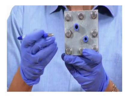
So, now we will look at this side of the hardware. You can see now there are two openings here one opening there and another opening out here. And this is basically the inlet the top one is the inlet and the bottom one is the outlet for one of the reactants it could be any of the reactants I mean we. So, one side of the cell will be receiving hydrogen and the other side will be receiving air or oxygen.
