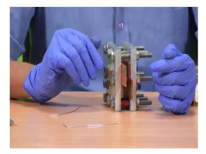
And therefore, you can put a torque wrench and then you know hold it on one side, so like this. So, you will hold it on one side and you will have a torque wrench on the other side and then you tighten it till you reach the correct torque.
