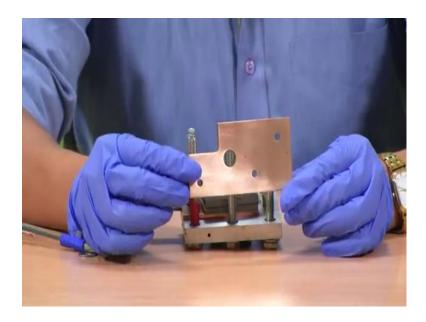
So, this is the one. So, this is a copper current collector. So, I am just taking it out here this is the copper current collector. So, it's made out of copper I just show you this current collector in different angles.
