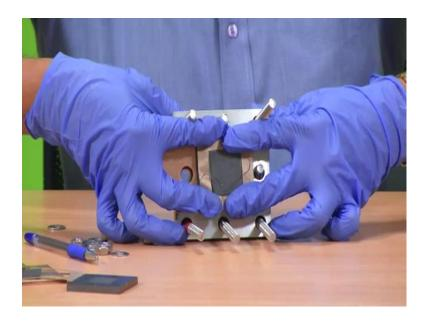
The silicone gasket is not visible because it is behind the the copper current collector and between the copper current collector and the end plate. So, that's why it is not visible, but you see the end plate, you see the copper correct current collector and you also see the gas flow channel all 3 of them are visible.
