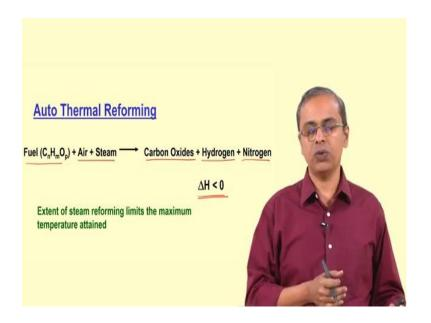
So, suddenly you don't need as much of heat exchangers etcetera relatively speaking because you now, take the fuel you mix both air as well as stream steam to the fuel both of them are being added to the fuel, and you take this complete mix and allow it to undergo this process of reforming. Again now, the output will contain carbon oxides it will have hydrogen, it will also have nitrogen because after all you are sending in air. So, this is what you do.
