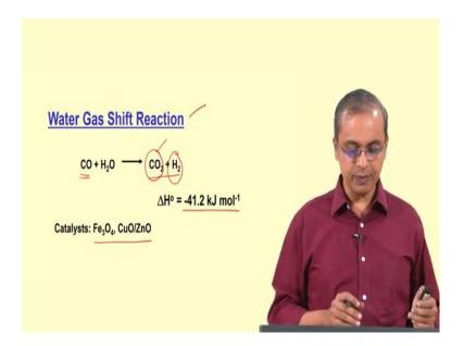
So, what we do is we enable you know two, other two more processes are often made available in a fuel cell reforming you know set up which then helps you to do cleaning of the gas stream cleaning from the perspective of reducing the CO content. So, one is called a water gas shift reaction which is what we have put here a water gas shift reaction which basically takes CO and gives it an opportunity to react with water moisture in this case and then that converts that to  $CO_2$  plus hydrogen.
