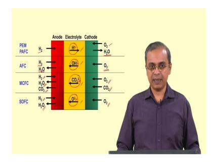
In the table that you see here for the various fuel cells the you at this point I only put the abbreviations down here, but they correspond directly to the types of fuel cells we saw previously. You can see here what reaction happens at the anode or what reactants arrive at the anode or what are possible reactants that can be used at the anode, what is the ion that goes across in the electrolyte and what are the possible reactants that are available for you at the cathode.
