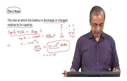
So, now I also mentioned there is something called a C-Rate ok. So, this is the rate at which the battery is discharged or charged relative to its capacity ok.
