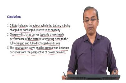
So, in conclusion we see that there is something called a C-Rate, we saw how the battery testing is done and in that context what is C-Rate it C-Rate indicates the rate at which the battery is being charged or discharged relative to its capacity.
