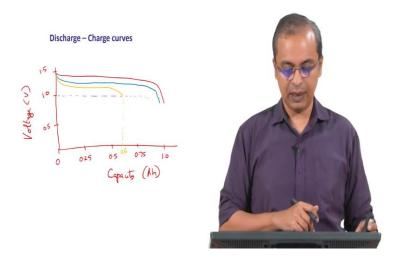
I will have again voltage here and I will have capacity. So, I have 1 ampere hour. So, this is 0 this is 1; so, this is 0.5 0.75, 0.25. So, this is capacity this is in ampere hours. So, the capacity is unaffected by what C-Rate you are doing right. So, the capacity of the battery
