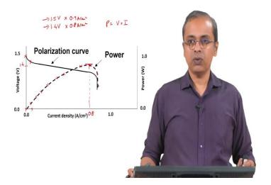
And from the same curve you can also find out the power curve; power as a function of current density. Because for example; when you are at open circuit voltage the current density is 0. So, therefore, the power is 0 V power is equal to V into I.
