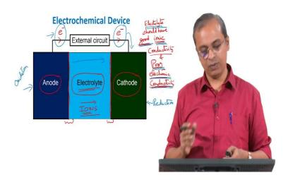
So, what are the major parts? As I mentioned there should be an electrode and an electrolyte, but for the battery to be complete you actually need two electrodes and an electrolyte ok. So, one electrode we refer to as the anode, and the other electrode we refer to as the cathode and in the middle there is the electrolyte.
