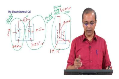
So, now, the electrochemical cell what we do as we saw here is that you have this anode and cathode and so, you can have a whole bunch of anodes and cathodes. So, you want to create a situation where you understand what will happen when you take one anode, and put it in or one material and connect it to another material with some electrolyte in the middle, you want to understand what will happen right.
