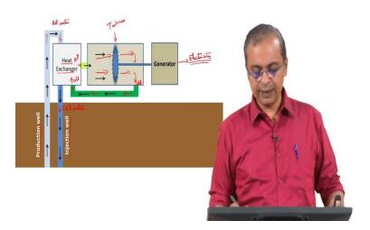
So, for example, it would look something like this. Again you would have a production well. So, from this you pick up the hot water and it goes into a heat exchanger. So, this is very important. So, we have a heat exchanger that is out here. So, in this heat exchanger this water enters hot.
