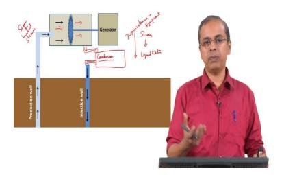
So, what we do is we put in a condenser. So, what comes out is actually sent into a condenser ok. So, here it is allowed to cool down further till it becomes liquid water ok. So, it becomes liquid water and then it is sent into this injection well ok. So, this is what is done. So, this may not seem like much. So, you would say, so what I mean you have you anyway across to the turbine.
