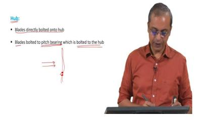
Then we will look at the hub, the hub if you go back to our diagram here this is the hub this part here is the hub okay. So, this is the central part of the wind blade arrangement.
