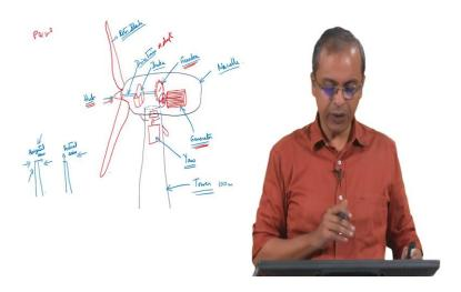
So, much of the design of wind turbines you know strongly acknowledges this aspect that the power is proportional to V cube and therefore, both in terms of cite, citing of the wind turbine as well as the general you know stature of the physical stature of the wind turbine is designed specifically to take advantage of higher wind speeds and therefore, those structures are typically pretty tall. So, that's something that we would have to keep in mind okay.
