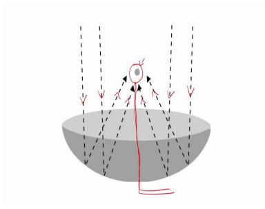
On your screen you see a parabolic dish, a parabolic dish is a way in which we are concentrating heat to a point that you see out here and basically its it is a parabola and then. So, the incoming radiation reflects of the surface of the parabola, and concentrates to the point which is its focus.
