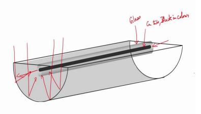
This is a parabolic trough as supposed to a parabolic dish that we previously saw. So, here it does concentration in the form of a linear concentration. So, along this line which is the tube that you see here, you have the concentration that is occurring and incoming radiation reflects of these surfaces and goes to this tube. And in that process it heats up the tube, you can again see two concentric tubes here, the inner is the black end copper tube and outer tube is glass.
