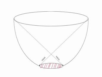
I am showing you this in the form of a trough here, you can also consider a version for it which is sort of a in the form of a dish, but this is still the non imagining concentrator, here you set it up such that the overall image could form anywhere here in a smeared sort of fashion and therefore, no there is no specific image being formed, but the energy is being captured. So, this is again a non imaging concentrator.
