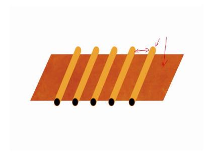
These are the parts of a flat plate collector you can see here the copper sheet. So, that is the your starting point on these are going to be placed a series of copper pipes, which will be placed and therefore, any solar energy that comes onto the copper sheet is then distributed to the pipes closer to it.
