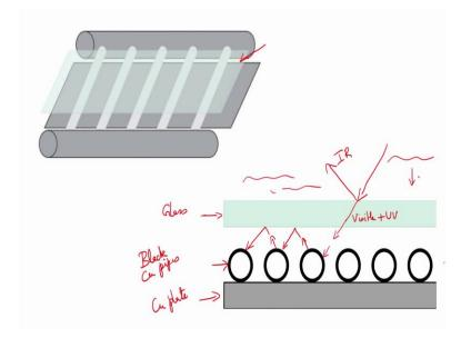
But you would actually need to make it black so that the energy is absorbed completely and is not reflected away from this surface. So, it's the same schematic here shown in grey in fact, here just for ease of observation of what it is, but in principle it could be black in color. In addition to this complete set up we would also need a glass plate on top; which is what I have added in this schematic that you see here.
