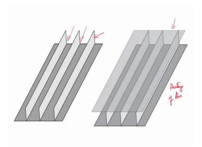
We looked at how a flat plate collector can be used for heating air and so, this is an implementation of how it will be used for heating air. You will notice that the main difference between the flat plate collector used for heating water versus that used for heating air is that previously we had pipes; we now have fins.
