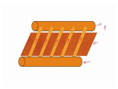
And then the hot water can be tapped from the tube on the top and the arrangement in the middle then does the heating of the water through the pipes that are there. And if you incline it such that the top side is inclined upwards; then the water flows in the direction that I have just pointed in this using these arrows; simply because the hot water will start moving upwards and cold water would remain at the bottom.
