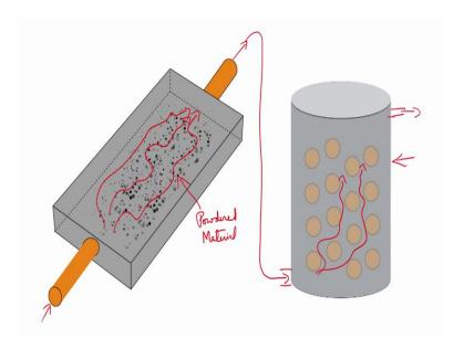
So, this a little extra pressure drop between the inlet and outlet, you have to account for that as you transfer this heat onto the air and use it for some application. Heating of air can also be done in a much more effective way; if you essentially increase the area of contact between the air and the surface that is hot. And we saw how by going from a tube to a fin you have actually increased the amount of surface area of contact.
