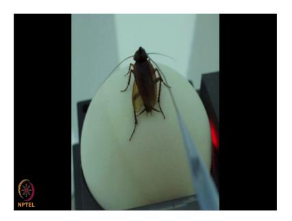
This is an example of a virtual reality applied to a cockroach. So, it runs on a foam ball that is suspended using air to make it nearly frictionless. And there is a wire there to study to do single unit recordings of its neurons and then it is presented with scenes visually on a screen and so, it will start running and exploring and you can control and
