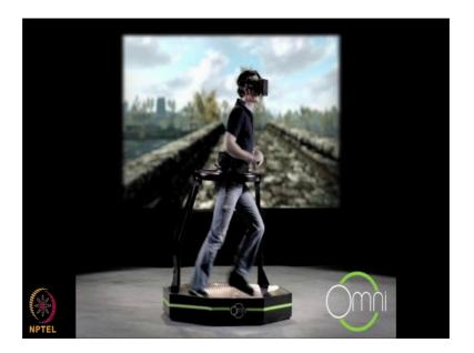
This is a picture of humans more or less doing the same thing as the cockroach. So, here they put on a virtual reality headset, but you could also have the surround screen; if you like and they are running around in some kind of omnidirectional treadmill dish; which was produced by a startup company recently.
