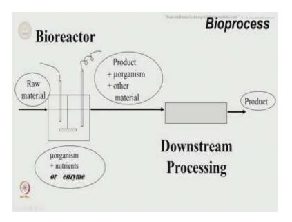
A bioprocess is something that is used to produce biological substances. It has two major aspects - the bioreactor aspects and the downstream processing aspects. Raw material flows into the bioreactor, it gets acted on by the microorganism in the bioreactor or the
