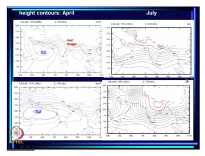
And this is very clearly brought out when we see the comparison between April where you have heat troughs sitting here. At 858 hpa you have a heat trough here and at 700 there is no trough at all because this is a heat rough. But in July you have a dynamic trough over this part and you see at 700 also very clearly the presence of a trough.
