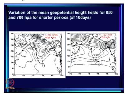
Now if we see on a shorter time scale, how does the geopotential heights field vary. Then we have this is the situation from 11th to 20th April, you see here a low pressure here, extending all the way here and at 700 there is no low pressure at all, in fact this part is a high pressure here. So this is a very clear signature of the heat trough again.
