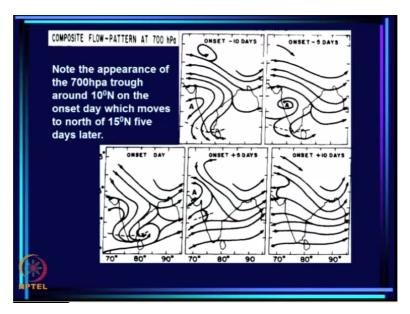
Now what happens to the 700 millibar trough 700 millibar onset -10 the trough is somewhere here. Remember 700 millibar trough is important because that delineates the TCZ or the dynamic trough and then this is the onset -5 days. This is onset day you see the onset day the trough is sitting right over Kerala here and onset +5 days it has already moved north to Mangalore or so and onset +10 days it has moved further north.
