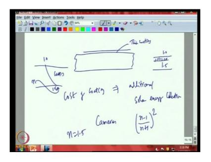
These are now routinely done in many devices, a thin coating does not fundamentally alter the transmission of the medium, but at same time reduce the reflectance, Hence more radiation gets in through the glass plate into the absorber. So, this calculation will help us to calculate to how much additional energy you will get in a solar collector, because doing thin coating and economic analyses to determine whether the cost of coating can be balanced by additional solar energy collection.
