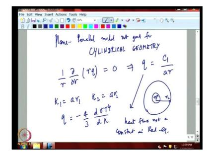
We notice that heat flux is not a constant in radiative equilibrium. This is the new feature of Cylindrical Geometry that even under radiative equilibrium, when there is no
