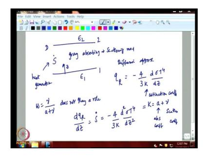
In this lecture, we take an example of solving slightly complicated problem of heat radiation transfer between two plates; surface one and surface two. This is emissivity, epsilon one; this is epsilon two and this is the gray absorbing and scattering medium in between Let us consider a situation where the heat generation is S dot and the depth of the plate is D.
