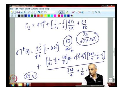
We can see clearly that, now there is a new parameter coming in; there is a heat generation into D by sigma. This will determine the importance of this term. This quantity is large; this term will dominate. We can essentially ignore this term. In that limit if the emissivity of the two walls is small, this will become large this term will drop out and it will be very simple quadratic expression here. But, on the other hand if the
