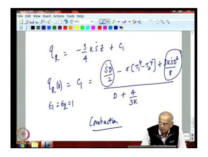
In the case of the present problem, radiative flux is not a constant. We can write this radiative flux as minus 3 by 4 K S dot Z plus C one, which we already highlighted. In this case because of the internal heat generation, heat flux is not a constant; it is varying linearly with Z. It is not so easy to compare the previous result. But, for example, suppose if we take q R Z is equal to zero; which could be a simple example. That is equal to C one and that we have readily available.
