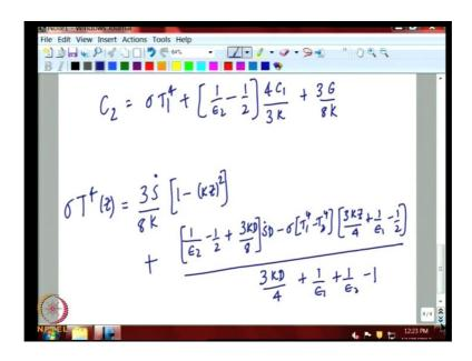
The C two will be related to C one and C two will come out as sigma T one to the power of four plus one by epsilon two minus one, , minus half, that is the boundary condition requirement, into 4 C one by 3 K plus 3 G by 8 K; where K is the extinct coefficient, not conductivity. We put all these into the final result, so that we get a feel for the final result. That will come out as sigma T to the power of four, a function of Z; this is equal to 3 S
