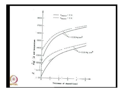
We can calculate this and we are going to show you the results of this computation through the result of the temperature of the gas as a function of thickness of the deposit. Now the deposit that is made outside of the tube has two influences. (Refer Slide Time: 27:31)
