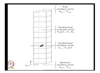
This is the model in which a series of volumes is of zero dimensions and gas slowly looses the temperature as it goes up, we solve this equation first and get the exit temperature, solve this equation so on in the vertical direction. This is one dimensional model, which will definitely be more accurate than the zero dimensional model, because accounts for the variation temperature along the path.
