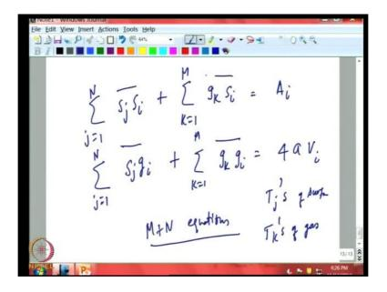
Our energy balance will tell us j 1 to N surface elements plus the M gas elements has to be equal to area of the surface A i and similarly, taking all end surface elements and interaction with gas elements and also interaction between all gas elements as equal to over a v i. These two equations put a constraint on the value of these exchanged factors and so we can solve for M plus N equation that we will have energy balance and solve for all the T j's of surfaces and T K of gas volumes.
