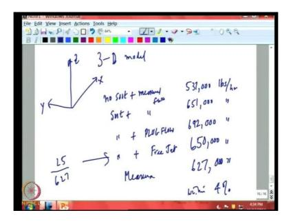
Quite clearly we need to go to the full 3 D model which accounts variation in the x y and z direction. So, all the three dimensions you account for, volume limits and so on. Then in this 3 D model if you have no soot and no convection, you get 531,000 pounds per hour. When we solve it, but no convection the value does go up to 651,000. This is plus measured flow.
