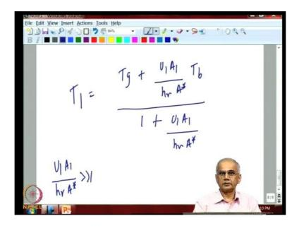
T l will come out as T g plus U 1 A 1 by h r A star into T b divided by 1 plus U 1 A 1 by h r A star. It is an approximate calculation. We can do a more accurate one numerically if we want to, but this highlights very nicely what the dominant issues are. Suppose the heat transfer
