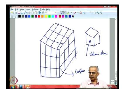
We look at the full furnace design. So, problem is truly three dimensional. If you think of this full three dimensional model, we can see that the furnace composed of large number of volume elements as well as surface elements. We need to extend the single zero dimensional model of Hottle to multiple dimensions this is called zoned model. Now, it is routinely used
