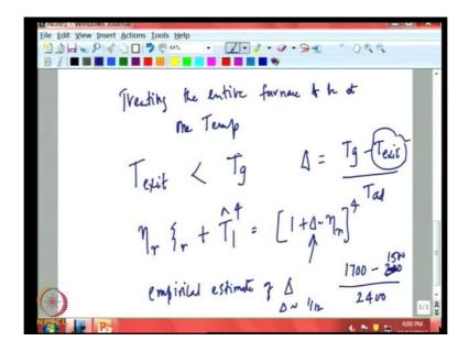
The others assumptions that has been made which could potentially cause large error is the fact that treating the entire furnace to be at one temperature. This is definitely not right because the exit temperature of the gas definitely will be less than the mean gas temperature of the furnace. This can be easily be accounted for if you assume that the difference in temperature between the mean gas temperature and the exit temperature divided by adiabatic term temperature.
