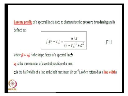
We saw that the typical collision broadening function is like this. In this function, nu 0 is the centre of frequency and alpha is the line width. This line width is a function of total pressure.
