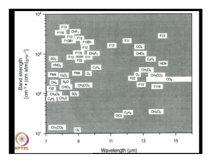
Now, here is the sample of various molecules which absorb and emit radiation. The wavelength ranges from 7 microns to 15 micron. We can see that there are large number
