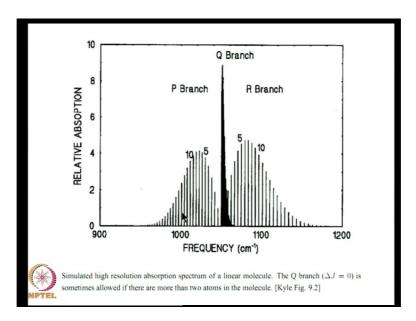
This is a typical vibrational-rotational band consisting of hundreds of lines. This is the problem one faces when solving problem in radiation that the absorption is the strong function of frequency or wave length and the variations are very rapid. For example, we have extremely high absorption at one wave length and immediately there is no absorption in the frequency between the two bands, between the two lines here.
