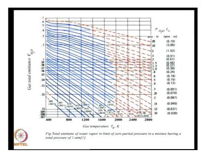
This is a typical behavior of carbon dioxide. Now, finally we need to estimate emissivity of a gas. We will ultimately integrate all wave length and get an idea of the emission. That is best done by using charts. But it is still a very useful tool to have a chart because we can do one sort of hand calculation to ensure that you have a good understanding of what is going on in this problem.
