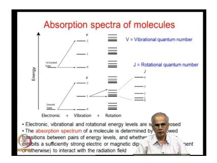
We saw that there are these vibrational transitions which come along with rotational transitions, which lead to three branches.
