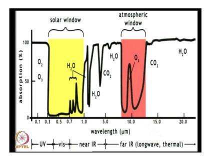
Now, this figure clearly illustrates the important difference between the solar region and the IR region. We can see in infrared region beyond around 0.7 micron, there is a lot of absorption by the atmospheric gases; H 2 O, carbon dioxide, ozone and so on. On the other hand below around 0.7 microns, atmosphere is almost transparent. Of course, this is the basis of the green house effect.
