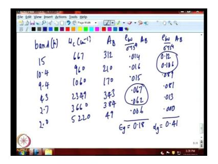
This is the centre of the band; it is centimeter minus 1. This is the band absorptance of the band. And, the contribution e b omega by sigma T g to the power of four into A B Then you have e b omega by sigma T s to the power of four A B. These two are the contribution for absorbed emissivity. Bands that are considered are 15 micron band, 10.4 micron band. Band is represented by the wave length by micron.
