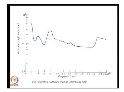
We have got a general picture of how the molecules behave. Let us see a few examples to illustrate. Here is the absorption coefficient of air at 12000 degrees Kelvin. Notice that, in comparison to what we saw for carbon dioxide, water vapor and so on, where the absorption coefficient has a very complex structure with wave length, here it is a fairly smooth function.
