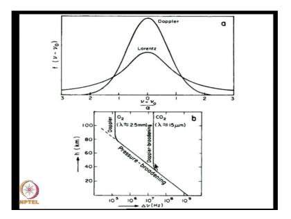
We can see that line width in this case increases linearly with pressure. That is why in the earth's atmosphere Doppler broadening dominates at low pressure above about 80 kilo meters, while pressure broadening is what we will see at the lower elevations for oxygen.
