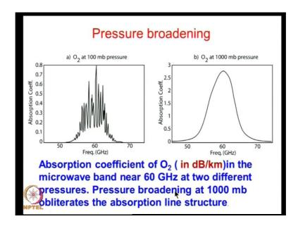
One more example we have given of oxygen absorption coefficient in the microwave for low pressure and for high pressure. We can see that, in the low pressure you will see all the high resolution fluctuations; while at high pressure, all of these get smeared out and we are getting a fairly smooth profile here.
