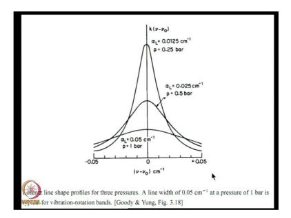
This figure shows the important effect of pressure on the line width. We can see that the line width which is only 0.0125 centimeter minus 1 at low pressure like one-fourth bar, as the pressure is doubled, the line width is doubled. Again the pressure is doubled, line width is doubled.
