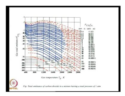
Here is the emissivity of carbon dioxide has a function of gas temperature. These are various path lengths going from 0.01 to 0.006. We can see that there is the region where the emissivity is not varying much, but there is another region where emissivity is falling fairly rapidly.
