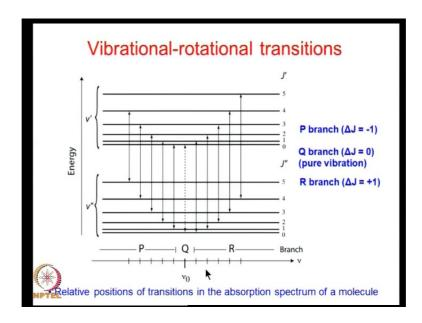
The Q branch which is purely vibrational transition the R branch and P branch, and in R branch the frequencies are higher, because there is both positive vibrational energy change and rotational energy change. In the case of P branch, the vibrational transition is upwards and rotational is downwards. So, the frequency is lower.
