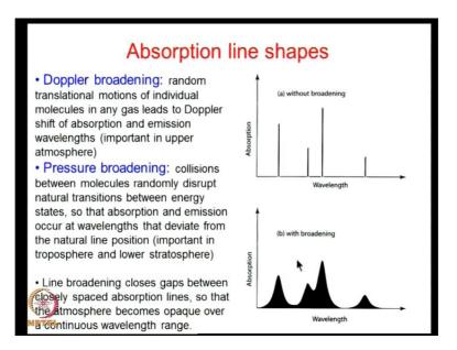
We saw the example of these lines as it exists and what happened to the lines when there is collision with the other molecules, which makes the line broader. The new feature of radiation transfer is, suppose we consider a medium containing carbon dioxide and nitrogen, carbon dioxide is the gas which absorbs infrared radiation; nitrogen does not.
