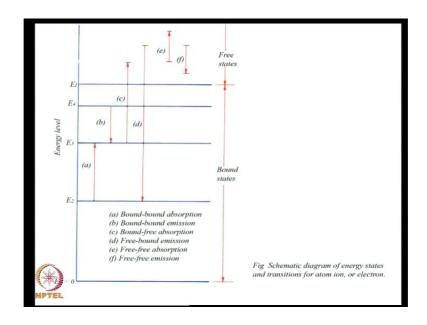
In the case of gases, the vibration-vibration transitions that we saw are all bound-bound transition. That is, it goes from one bound state to another bound state. The energy absorbed is precisely fixed by the equation delta E is equal to h nu. On the other hand, if the temperature is sufficiently high, molecule can jump from bound state to free state. In the free state, the kinetic energy of the molecule can be anything. Hence, we absorb radiation continuously with no gap in between.
