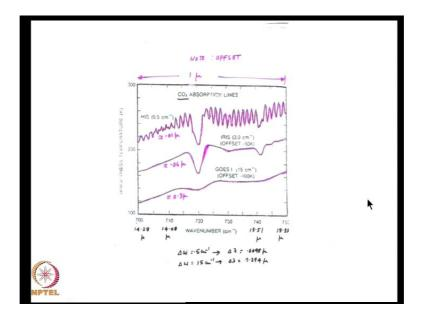
Lastly, we will see how the atmospheric measurement of carbon dioxide emission by satellites. The older satellite had extremely poor resolution about 15 centimeter minus 1. So, could not really resolve the carbon dioxide spectrum in 720 or 14 micron, 15 micron
