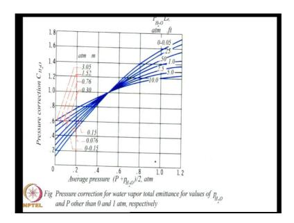
Here is the correction chart for water vapor, if it is not at the total pressure or one bar.
