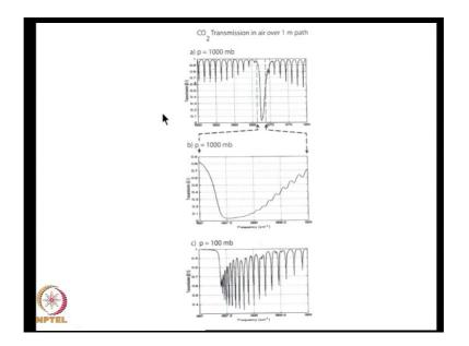
We show once again the impact of pressure; it starts with 1000 milli bar. We get the full carbon dioxide spectrum at 670 centimeters minus 1. Then we look at a close up of the absorption band right close to 667. We see that this thing has slight waviness. That waviness is there because of the lines. But these lines are not fully resolved.
