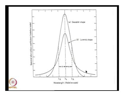
We saw the typical profile of the Doppler broadening and Lorentz broadening. Doppler broadening has a Gaussian profile. Hence, it steeply falls to 0, while the Lorentz broadening goes 1 over 1 plus x squared. So, it goes down with frequency at a much slower rate. We can see that we can have situations where in the Doppler broadening dominates near the centre of the line, while at the edge of the line, Lorentz profile dominates.
