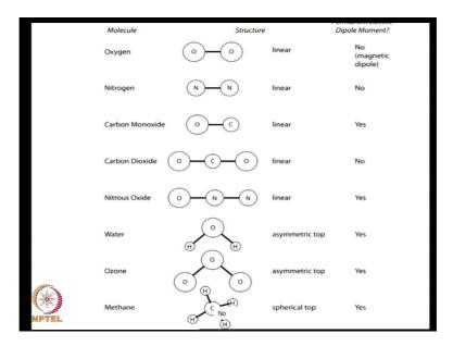
We saw examples of various gases. We pointed out that symmetric diatomic gasses like oxygen, nitrogen have essentially no absorption bands because they have no permanent dipole moment. When they vibrate they do not have a dipole to interact with the electric field. They do not absorb or emit radiation.
