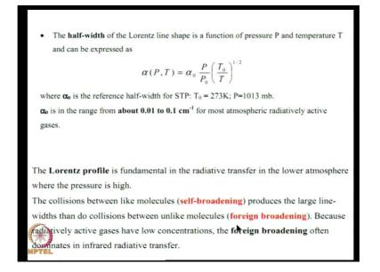
The line width depends on total pressure. If you increase total pressure by adding a non absorbing gas, we will change the line width. Hence, change the ability of carbon dioxide to absorb radiation. This is unusual paradox which we do not find in many other fields. That is, a molecule which does not absorb radiation by itself is able to alter the radiative
