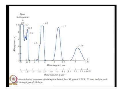
Now, let us take an example, of carbon dioxide. We saw that air is continuous spectra. Now let's look at the absorption band of carbon dioxide at a fairly high temperature 830 Kelvin; typical situation kind of furnace at a fairly high pressure and the gases at ten atmospheric pressure and in a container of the length scale 38.8 centimeters.
