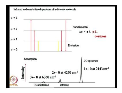
Then we saw that if gas temperature is high, the transition can occur instead of one level, it can be two levels and these are called over tones. These are important in high temperatures, especially in furnaces.
