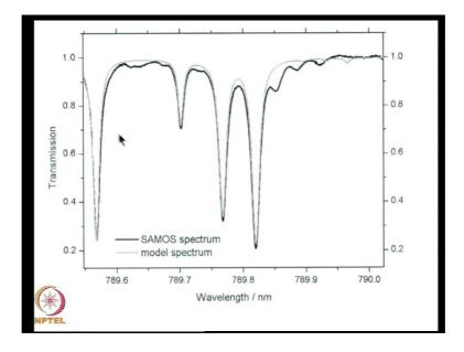
So for accurate estimate of fluxes, it is important to use as high resolution as is practically feasible. Now we look at the same spectra again, instead of 8 nanometers looking at only 0.4 nanometers, very high resolution. This one comparing the absorbed spectrum with the simulation spectrum, showing that the simulations have reached fairly high level of accuracy. It is able to identify each line in this band and showing a large spacing between the lines.
