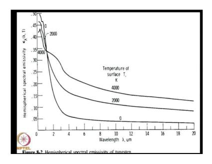
This is good use full information we get from this report that gray surface approximation is good. If the temperature different with the two plates not large, less than 1000 degree Kelvin, but as we go to a higher temperature difference, the gray surface approximation becomes worse and worse.
