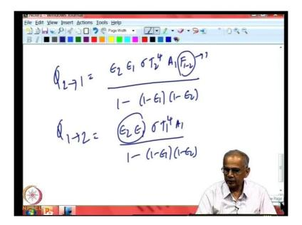
So, the radiation that is emitted in this quadrant only will bounce back between 1 and 2, only radiation coming or the other direction will go. So, even from here this is a normal emission, this is tangent and the tangent emission, will come back to 1 and will not go to 2. So, once we have realized this, we can see clearly that we can write down the final expression for Q 2 1, as equal to being infinite series summation and A 2 F 2 1 is A 1, F 1 2 and F 1 2 is 1 and F 2 is 1.
