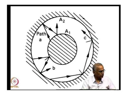
If that is case one can still extend the techniques, we have developed for diffuse isotropic reflect in emitter to an enclosure with the few surfaces which are spectral. That is what we are going to a focus on, which is spectral. That is what we are going to focus on. Now, let us now take some simple examples first to highlight the role. Now, first example let us imagine two cylinders or two spheres, now to mentally do the ray tracing.
