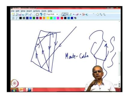
So, suppose we have an enclosure and radiation came as shown in the above figure. We have to follow that radiation which is reflected. We have to follow the ray through all the reflection. We can do it today with a computer. This method of tracing the ray and following the photon till it is absorbed. We start with the photon emitted by some surface and follow that photon through after multiple reflections until it is absorbed and we do this same procedure for maybe a million photons.
