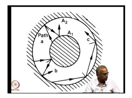
So, the surface is specular than the final answer looks like that between parallel plates. So, when both the surface here is specular then the heat transfer between two cylinders or two spheres looks like heat transfer between two parallel plates. We had already used this idea, when we looked at the Dewar flask problem. We did not explain it as to why we used that formula.
