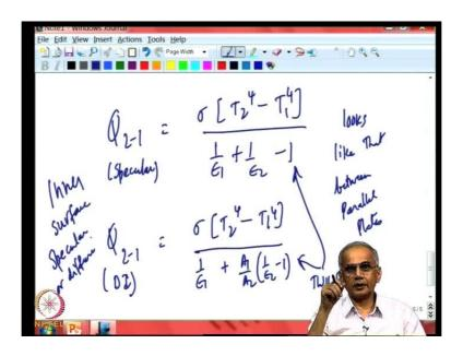
That is to remind you the difference between this result and result for this was specular surfaces. This is for D I surface two cylinders, this was what we got we earlier D I surface
