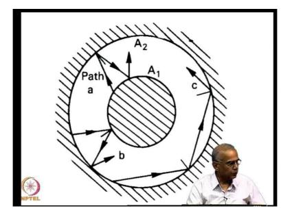
The fraction which is reaching 1 the inner cylinder or inner sphere reflects between 1 and 2. Once it hits 1 and 2 till it is absorbed. The other fraction 1 minus F 2 1 is only reflected between 2 and 2. So, let us go back to the picture to make sure that we understood it. So, sigma T 1 to the power of 4 a 2 F 2 1 is this one and sigma epsilon 2 sigma T 2 power of 4 to 1 is F 2 1 and is this one.
