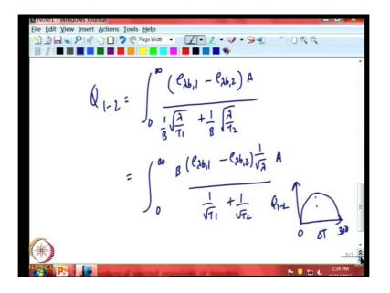
On neglecting this term be the expression we got between two parallel plates was, e lambda b 1 minus e lambda b 2 into A divided by 1 by epsilon lambda1 which goes as root lambda by T 1 1 over b plus 1 over b root lambda divided by T 2 and root lambda is common to them. This can be simplified to write as, 1 over root lambda goes above and below we have and we can write A above, then take also B above nothing but 1 over root T 1 plus 1 over root T 2.
