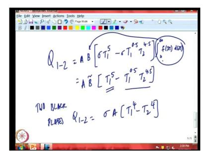
What will happen is we get B here and actually we get A B delta, actually to write down the whole thing B and we will get T 1 to the power of 5 sigma T 1 to the power of 5 minus T 1 to the power of 5 sigma here T to the power 4.5 and what we are inside in integral 0 to infinity, this integral which is function only of lambda T d lambda T. This is a number which can be evaluated very easily and we just combined with this we did earlier and we call it B delta along with sigma.
