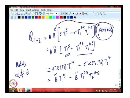
We now write this very simply as, epsilon function of T 1, T 1 to the power of 4 into sigma minus sigma alpha a function of T 1, T 2 into T 1, T 2 the power of 4 this how it should be because, in the case of metals we must recall that alpha is not equal to epsilon. That was the fundamental result, we are derived that metals being non-gray, we cannot assume that the total hemispherical absorptivity is equal to total hemispherical emissivity.
