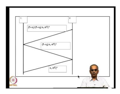
The simplest way to understand the heat transfer between the two surfaces is to do a simple ray-tracing, the radiation emitted by surface 1 reaches surface 2; is partly absorbed; the remaining part is reflected and it is reflected back to surface 1 again. One can add up the total number of photons arriving from 1 to 2 and being absorbed at 2 as an infinite series; the direct contribution after 2 reflections, 4 reflections, 6 reflection so on and this standard ray-tracing technique.
