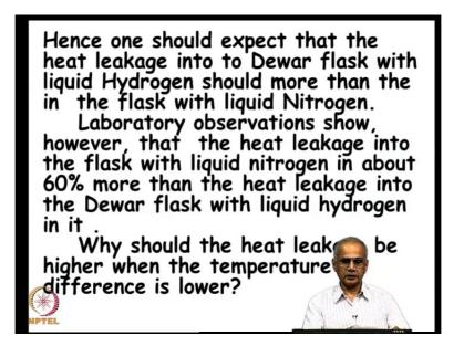
Laboratory observations show that, heat leakage into the flask with liquid nitrogen, which has a lower temperature difference, is about 60 percent more than the heat leakage into the Dewar flask which contains liquid hydrogen. The question is, why should heat leakage be higher, when the temperature difference is lower. This is the issue we want to address and understand, from radiative heat transfer.
