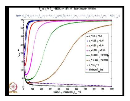
We can see, that as the cutoff wavelength is increased, from around 10 microns, all the way to a 1000 microns, the minimum temperature which is a the dot line here, goes on decreasing; and ultimately, will reach 2.72 degrees Kelvin, asymptotically. But before that, notice this interesting feature, that if your surface had, let us say the green one, emissivity only 0.0001 in the solar region, but a very high emissivity in the region beyond lambda c; then, we see that, we get this kind of curve.
