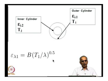
In the new derivation, now, we take into account the fact that, the spectral emissivity of metals, because the outer surface of the inner cylinder of the Dewar flask and inner surface of outer cylinder, are both silvered. Silver is a metal and for that, we can assume that emissivity is a constant times temperature of that surface divided by lambda to power of 0.5. This is the
