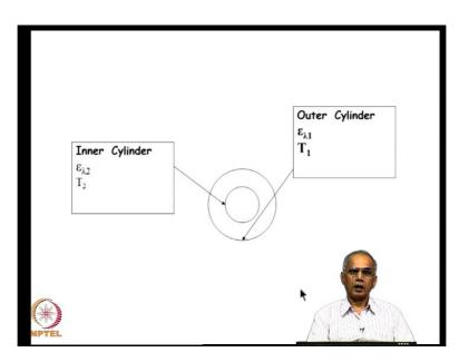
To do that, we treat the Dewar flask as a simple, two parallel cylinders. The inner cylinder is at temperature T2, which is close to the boiling point of hydrogen or nitrogen and the
