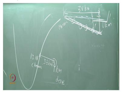
To reach 1 kilometer depth you have to go 38 kilometers. So, which means if this is your marina, it is very gentle. This 1 kilometer takes about 38 kilometers. So, if you want to have a power plant based on Vortech you should be able to lay your pipe here right and then you should be able
