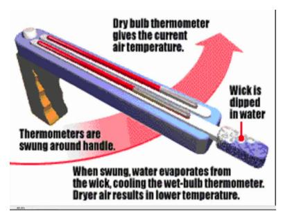
So this is the this is the sling psychrometer used for getting the wet bulb temperature. The dry bulb temperature gives the current air temperature. What is the air temperature now? The air temperature is always measured in shade. It would not be measured in the outside. It has to be it will give some wrong reading just like you take coffee and then check your body temperature okay. It has to be measured in the shade and all these are measured 2 m above sea level, 2 m above the ground okay.
