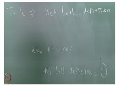
The difference between the dry bulb and wet bulb temperature, suggest a name for this, the difference between the dry bulb and wet bulb temperature, there is a technical name for that. That is called the wet bulb depression. It is the bulb is not depressed right. When RH is equal to 100% wet bulb depression equal to very good that means you have understood. So we agree that the wet bulb temperature is also an indicator of RH or the moisture content in the atmosphere okay.
