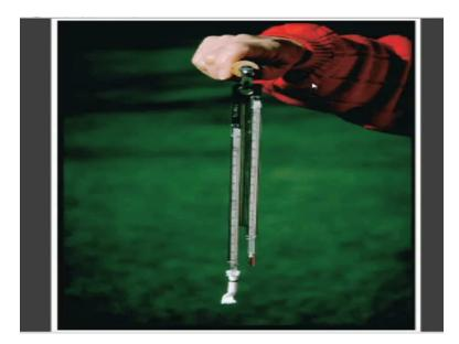
Okay, are you able to see this? So this is another. So where is the wick? It is here, the wet cloth is here and he is swinging it here right. He is swinging it here. Are there 2 thermometers? What are they giving wet bulb and dry bulb okay so this is the sling psychrometer okay.
