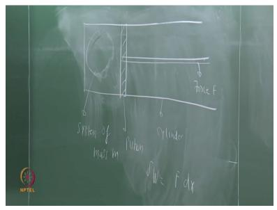
So, consider a cylinder and piston arrangement. System of mass M, okay so, you have got a air combustion, gases whatever you want, okay. This is your piston. So, the piston is moving either you are compressing or it has got high pressure it is moving in the other direction, okay. So, when force moves by a distance that is work, okay. dW is f dX.
