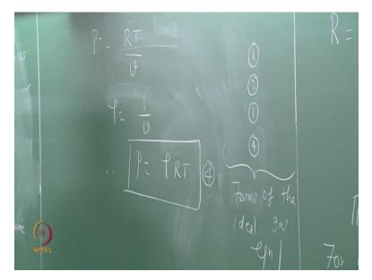
So, the ideal gas equation is PV = m RT, okay, Pressure, Volume, Mass, the gas constant, okay. Please forget that PV = NRT and moles and all that, okay. Sometimes it may be useful in the thermodynamic in chemistry and all that. But as an engineer I hate PV = I am sorry to say hate that PV = NRT, right. Mole cannot 1 kg is easy to comprehend, okay. So, your teachers have taught PV is = NRT, please remember that if you want. There is no problem. R is the gas constant what is, what is this R?
