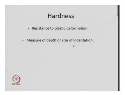
Now, what when we say about hardness, so mechanical properties many times refers to hardness or strength, what you mean by hardness, it is the resistance to plastic deformation, that means how much strain it can take before it become non-linear, so that is called the hard material. That means, it will remain, it shows resistance to plastic deformation, so this can be measured, the hardness can be measured by the depth or size of indentation.
