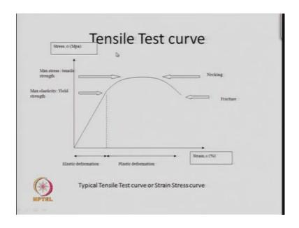
Now, in the tensile test curve you can get a maximum elasticity is what you get in the linear portion and then the curve become non-linear, so this point here is this is the region where you have the elastic deformation. So, this access the x access plots the strain and till this value of strain you have an elastic deformation, where the yield strength the stress is directly proportional to the strain and this point is called the yield strength, because beyond this it is no more linear.
