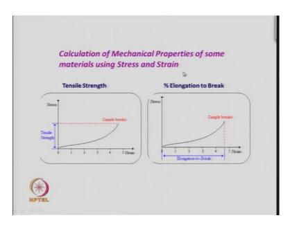
Now, mechanical properties if you want quantitative, so you measure for example, in a stress strain curve, most of the times we are measuring stress strain curves for materials when we are studying their mechanical properties. So, here you are plotting again stress and you find that the stress varies like this and beyond this there is no plot, because the sample has broken here.
