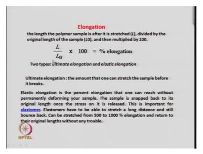
And this percentage elongation is also what we measure which is given by the length, by the initial length multiplied by 100. So, instead of strain which is given as ratio you may also define it, in terms of percentage elongation, where you multiply the final length divided by the original length into 100. So, you can have two types of elongations, the ultimate elongation and the elastic elongation, the ultimate elongation is that amount that one can stretch the sample before it breaks.
