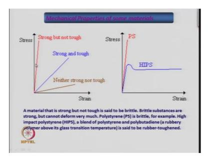
Now, if you see different material, so suppose this is material a, this is a material b, this is a material c, now the differences is for example, in this case it is very sharp the slop, so for very high stress the stream is very small. So, it elongates to a very small extends even though you have given a large stress and that means, it is strong, but it is not very tough.
