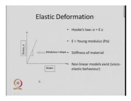
Now, normally we plot for any elastic deformation, you plot the stress verses strain and since it is elastic, it is normally liners, so there will be a straight line between the stress and the strain. And this slop of this stress strain plot will give you the modulus and this is given by Hooke's law that, this linear portion which is called the elastic deformation follows Hooke's law, where the stress is proportional to strain.
