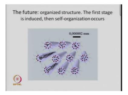
So, this is the future is to organized the structure, so you have to make a rope with all these fibrous things organized like this and that will give you the strength of this bundle. So, each of this nano fiber should be aligned in a particular direction such that, it appears like this bundle and then many of this bundles together will give you the real strength or power for the rope to carry very, very heavy loads.
