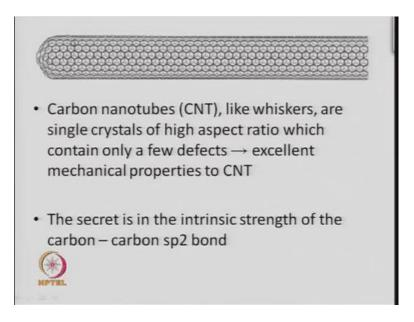
Now, these nanocrystalline materials like carbon nanotubes have been discussed in the literature to large extent, lot of studies have been done on the mechanical properties of carbon nanotubes. Carbon nanotubes are nothing but if you takes single sheets of graphite, so one sheet of graphite is made up of hexagons of carbon and if you roll them, then you can get this a nanotubes.
