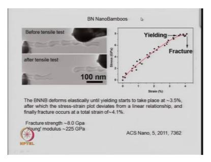
Now, this has not only been seen in carbon nanotubes, but there are other material for example, boron nitrite, boron nitrite has slight similarities with carbon nanotubes.
