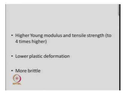
So, when you say a higher stronger mechanical properties, for example you will have much higher young modulus and tensile strength in nanoparticles. Sometimes it may be 4 times higher than the same material, which has got micron sized particles, it will also show lower plastic deformation compare to micron sizes particles and will be more brittle. So, the nanoparticles will be the material made of nanoparticles will be more brittle.
