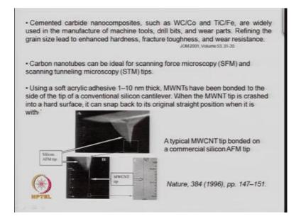
So, these some examples of these cantilever tips, so I showed this is a cantilever, ((Refer Time: 50:43)) this is the surface, and this is the cantilever tip. Typically in a AFM the laser light is guided on the back side of the cantilever, which is deflected on to a photo diode and any change in the position of the cantilever tip, can be determined by the deviation of the reflected beam of the laser.
