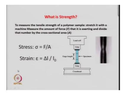
You have to measure these stress and strain, etcetera, so how do you major the tensile strength for example, you have a polymer and you stretch it with the machine and then major the force F that it is exerting. And if you know the cross sectional area then F the force divided by the area will give the stress and strain is as we defined just before is the deformation length delta l divided by the initial length l naught, that gives you the strain.
