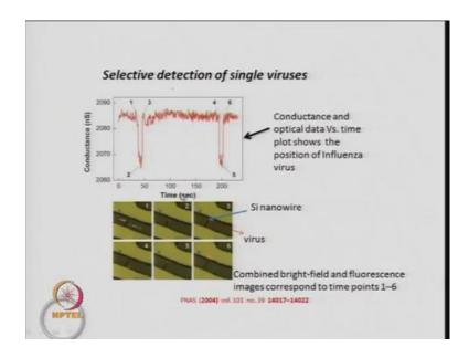
So, this is what is being shown by single wire detection by nanowires. So this is a silicon nanowire and there is this red dot is the virus. So, when that virus is on the wire that is
