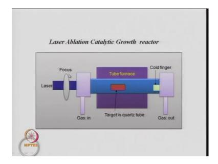
This is the setup which you use for the laser ablation technique. So, you have a furnace and you have your material on which the laser has to be focus so your target is in a quartz tube and you have the gas, which is the semiconducting gas which is going to be around that target.
