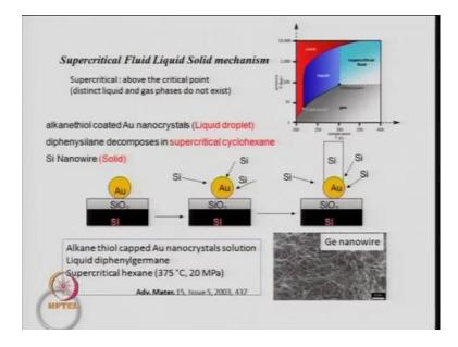
Now, going into another methodology of making nanowires, this is called the supercritical fluid liquid solid mechanism. So, supercritical fluid, what are supercritical fluids? So, basically anything in physical chemistry or chemical engineering, you may be aware that liquids which cross a certain critical point in the phase diagram.
