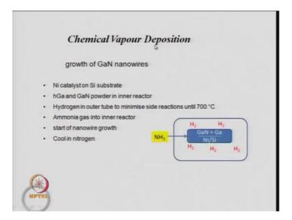
The other technique, which is of importance was the chemical vapor deposition and here for example, I have shown you the growth of gallium nitride nanowires, very important material where, you have a nickel catalyst on a silicon substrate. So, you have a nickel catalyst on a silicon substrate, and you have a gallium, and a mixture of gallium and gallium nitride powder in the in a reactor.
