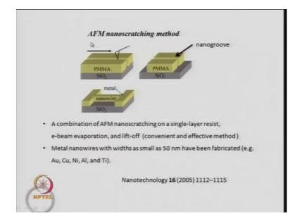
Now, another method is using an atomic force microscope. So, in atomic force microscope you know that there is a cantilever, and at the tip of the cantilever you have this kind of a tip, which is normally made up of either tungsten or platinum or iridium. There are lots of different types of tips which are available.
