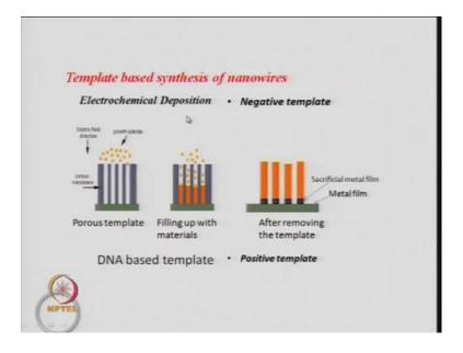
There are other methods which is the template method we discussed, where we use the electrochemical methodology of deposition, this is a negative template method. That means wherever the template is there so this grey one is your porous membrane which acts as a template so the voids get filled with the growth species which you want to make nanowires.
