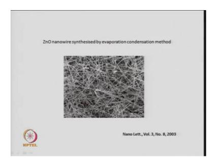
Now, this is a TEM picture to show you the growth of zinc oxide nano wire zinc oxide is a semiconductor. You see you have large bunch of nano wires, but they are not aligned along around one direction which we were we just mentioned that the direction of growth of nano wire cannot be controlled. You make a large is like a forest of nanowires made by evaporation condensation method by which has been published in a journal which is called nano letters in 2003.
