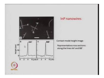
So, either you directly you can measure the size using what is called the z movement of the AFM or your measuring basically the z the direction which is also the height using a AFM.
