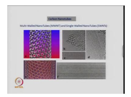
So what we discussed briefly was about different types of nanotubes, both multi walled nanotubes and single walled nanotubes. And these nanotubes as you see are made up of hexagons of carbon, and when these nanotubes the cylindrical part has to closed, they have to have pentagons and heptagons.
