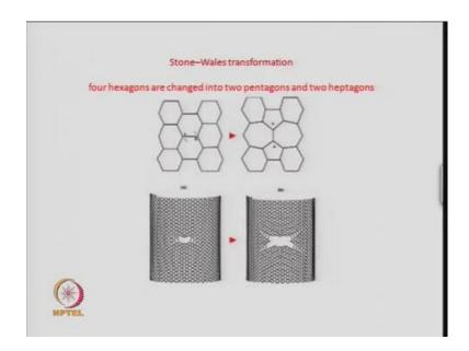
Now, here one of the defects which is very important in carbon nanotubes or most of the carbon structures is that, if you consider 4 hexagonal rings next to each other, so if you look at 4 hexagon rings in the graphene layer, you have all, the entire plan is made up of these hexagonal rings.
