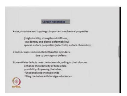
So, you will have these caps, which are different compare to the cylindrical part which has mainly 6 membered rings of carbon. So, you have 6 membered ring of carbon in the cylindrical part, whereas the caps which are part of the C 60 or C 70 or C 80 molecules will certainly have some pentagons. So, towards the end of the nanotube, you will have these pentagons or heptagons, which is necessary for the curvature of the nanotube.
