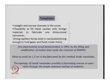
So, other than that, now nanotubes as you know if it is closed there is hollow space inside the nanotube. So, can it act as a template? That means, you have this hollow thing and then if I fill something, it will take the shape of the carbon nanotube.
