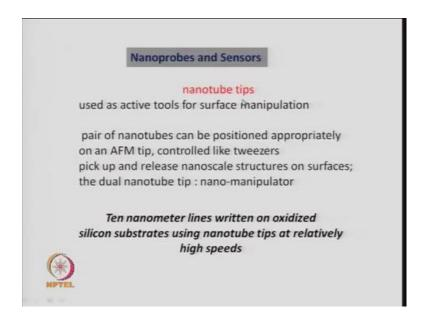
As we discussed or look at the surface of these biomolecules, but you can also use these nanotube tips for manipulation for surface manipulation, like a tweezer. So if you have instead of one nanotube, suppose you have a pair of nanotubes, two nanotubes which are placed appropriately on an AFM tip, then you can bring this pair of nanotubes very close to say a biomolecule or some nanoscale structure on a surface. And then you can hold
