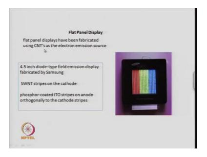
But, people have made flat panel displays. For example, using carbon nanotube as the electron emission source, people have made a 4.5 inch diode type field emission display this was fabricated by samsung.
