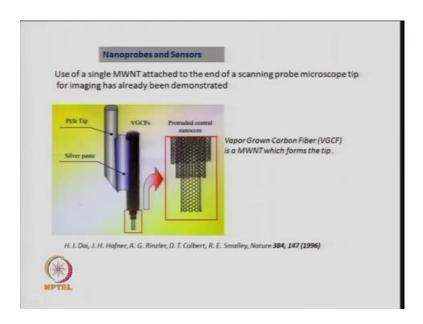
So, if you want to look at a nanoprobe of using a carbon nanotube, so you know there are a in all a scanning probe microscopes today, you have a tip and that tip can be made of many metals are used, like platinum or iridium. That is the tip which is found in most scanning probe micro scopes.
