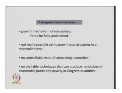
So, there are several challenges for carbon nanotubes, alike the growth mechanism of nanotubes is yet to be understood. And these structures cannot be controlled in exactly the way you want. Then, connecting these nanotubes is also not easy and still there are requirements for producing these nanotubes in large quantities. So, we will save, we will stop here today and we, I hope that you got a good idea about carbon nanotubes and its properties and applications.
