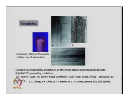
Now, if you look here this is a schematic diagram so you have these say 1 carbon nanotube and there is another wall of the carbon nanotube, so this may be called a double walled carbon nanotube and inside the hollow part you have filled with something.
