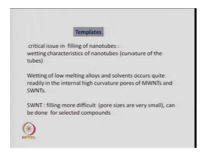
Now, the critical issue in filling the nanotube, when you fill nanotubes is the wetting characteristic of the nanotube. And that depend on the curvature of the nanotube. So, wetting of low melting alloys and solvents occurs quite readily in the multi walled nanotubes and single walled nanotubes.
