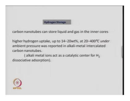
Now, you can also store liquid and gas in the inner cores, so you can store hydrogen as we discussed and you can also store liquids. So, higher hydrogen uptake up to 14 to 20 weight percent under ambient pressure is possible, if you have alkali metal intercalated in the carbon nano tubes. If you have just carbon nanotubes then, you can take around 4 to 5 weight percent of hydrogen.
