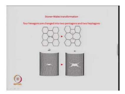
But here we discuss one of the important defects or an important transformation of how ideal hexagonal layer can generate instead of hexagons, pentagons and heptagons and which lead to curling of the graphene layer.
