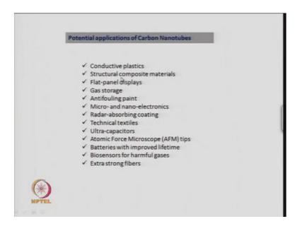
Now, a large number of applications I have listed here in industry. So, starting from conductive plastics, structural materials, because these are very mechanically strong. Flat panel displays, this comes from the unique electronic properties of a carbon nanotubes. Then, we will discuss about gas storage and several other properties, using tips made from the carbon nanotubes in AFM.
