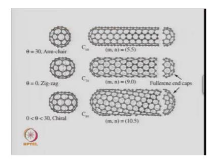
And this, that angle as we discussed earlier is a for theta is equal to 30 which is chiral angle, you can cap with a C 60 molecule. But of course, if these this cylindrical part is made up of a chiral angle which is different like if theta is 0, then you have C 70.
