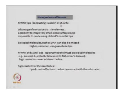
So, using these multiwall nano tips, if they are conducting then you can use them in STM because you know in STM the surface is metallic and there is a tunneling from the surface to the tip and the tip has to be conducting in STM. And in AFM, you can use this kind of tips to study the changes in the atomic force.
