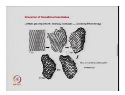
Now, how do these nanotubes form? So, what is the mechanism of nanotube? Though the mechanism is not exactly understood, but it is known that defects are very important for formation of nanotubes. So, people have done computer simulations and other studies, where if you take a single graphene layer and run the simulation, then with time you see that this single graphene layer will generate defects which are not hexagonal.
