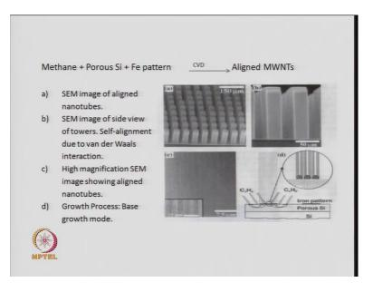
Here, you can see a picture of the CVD method on a substrate. The substrate is porous silicon and you are passing methane gas. You have iron pattern on it as a catalyst. So, these are your silica to the porous silicon and you can see the align nanotubes. This is the side of the towers and this is the SEM image to show the aligned nanotubes.
