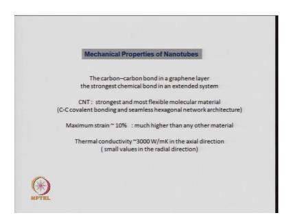
From electronic properties, if we look at the mechanical properties of carbon nanotubes, there are also excellent. The carbon-carbon bond in a graphene layer, have carbon-carbon bonds to form six membered rings, and then these six membered rings are then connected to other six membered rings, and it forms a layer or it forms an extended system.
