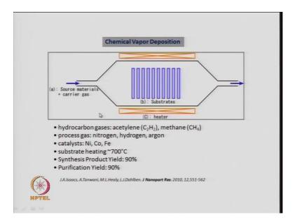
In the chemical vapor deposition, you use hydrocarbons, like acetylene or methane. It is passed through a chamber, where there is a substrate, on which you want the deposition to occur, and there is a heater to heat the substrates. So, the temperature of the substrate is around 700 degree centigrade. So, what you are passing, is the source of carbon here, is a gas which is a hydrocarbon and typically, you use acetylene gas or methane gas for the carbon to deposit on the substrate.
