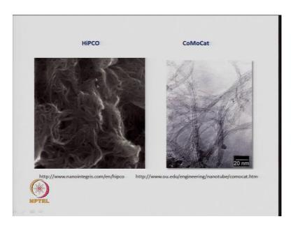
This is a TEM of the carbon nanotubes, made by the hipco method. You can see all these curvilinear form of carbon nanotubes. By the CoMoCat method, you can see much better quality of carbon nanotubes compared to the hipco method. Here, you are using a catalyst of cobalt and molybdenum and here you are using iron pentacarbonyl as catalyst.
