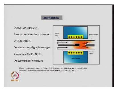
Using laser ablation which was developed by Richard Smalley, at tries university in Texas, USA in 1995. What he did was, he took this graphite target. You take a piece of solid graphite and you use a laser beam on top of the graphite target, which is heated by a
