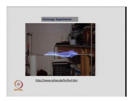
This arc discharge method, it is a high temperature method. This is a typical discharge which is taking place between the two electrodes, and during this discharge, which is between graphite electrodes you have, and then the deposit is on the cathode and from that deposit, you can extract the carbon nanotubes.
