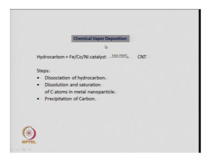
In a typical CVD method or the chemical vapor deposition, you have the hydrocarbon, you have the catalyst and around 700 degree centigrade, you get CNT. The steps which occur is, first, the hydrocarbon dissociates and then it dissolves on the metal catalyst, and then it saturates the carbon atoms in the metal nanoparticle and finally, you precipitate, reprecipitate carbon in the form of nanotubes.
