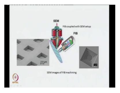
It is impractical for mass production it has high cost. As you see the equipment is quite complex because we have several lenses apertures and blanking devices within this chamber. You have detectors for SEM and again several lens as electromagnetic lens is built in the SEM. So, this whole equipment becomes very expensive for making patterns on substrates. Now, we discussed the advantages as well as the disadvantages of e beam lithography.
