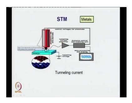
The STM again has a tip, but now you do not measure forces, you measure tunneling current on the forces right. This allows you to understand the topography of the surface. This is a typical scanning tunneling microscopy, where you measure the tunneling current and understand the topography of the surface. However now you are going to use the same tip of the scanning tunneling microscope and we are going to measure. You are going to make patterns on the surface.
