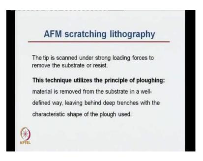
A very strong force is applied strong loading force is applied to remove the substrate or the resist which is on top of the substrate. That will remove some substrate atoms or molecules. This technique is like ploughing, like in a field in agricultural land we have seen how people plough on the field and you leave patterns on the ground. This is typically like that. So, you have an AFM tip and you bring it with lot of force. So, lot of load on the surface and then you move the tip.
