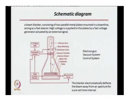
Now, another schematic diagram of this process of how a electrons are focused is you have this chamber which is an electron gun. So, in this electron gun electrons are generated because you apply a very high potential here. It is like a cathode ray tube you have a cathode a metal foil from which you can get electrons. These electrons traverse this region where you have something called beam blanking.
