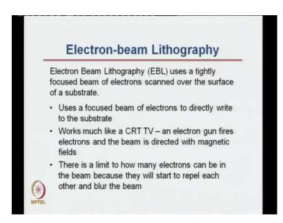
From the term electron beam Lithography, you can make out that you are going to use an electron beam to make patterns on surfaces. So, the electron beam lithography will use a
