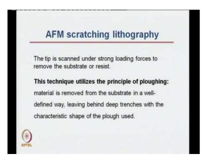
So, for this the most important thing is the substrate has to be modified to create the steps or the patches where you want the pattern to grow. Now, you can also use a scanning probe technique to make patterns by removing atoms from the surface. It is like etching away from the surface the term we are calling it as scratching. AFM scratching lithography that means you remove the atoms from the surface. So, the tip is brought on top of a surface at particular point where you want.
