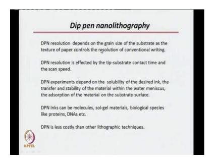
The resolution of the technique depends on the grain size of the substrate. So, if your substrate is very fine grained. Like if you write with ink on a paper if the paper has small grains which is very fine, then it will control the resolution of your writing. Similarly, if the substrate on which you are doing dip pen nanolithography, if that has very fine grains then your resolution will be high, but if you have very large grains then you will have very low resolution.
