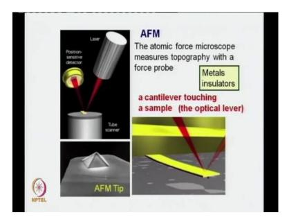
Here we are trying to make patterns on the surface. Basically an AFM all of you know that involves a cantilever and a typically you shine a laser on the cantilever. The cantilever if it has a deflection because of the surface will show up in the detector because the laser beam will move its position. From that you can calculate the force between the cantilever and the surface.
