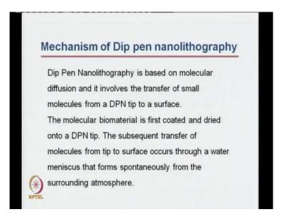
So, this is the dip pen nanolithography is based on molecular diffusion. It involves the transfer of molecules from the tip of the dip pen, which is typically an AFM tip on to the surface. How you do it is, first you take the molecular biomaterial. Normally, it is used a lot for bio nanotechnology or bio sensing etcetera.
