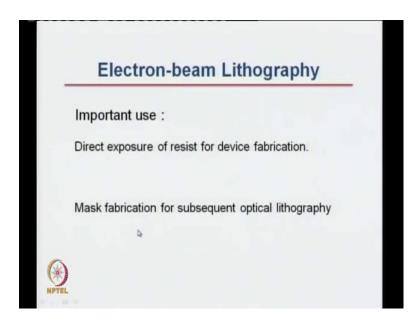
Now, the use of these kind of ion beams or electron beam lithography, is that you can directly expose the resist for device fabrication. We discussed what are resists in our previous lecture. Here you can directly use the electron beam to make devices. You can also make masks based on electron beam lithography, which can subsequently be used for optical lithography.
