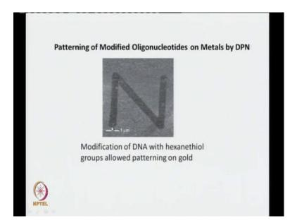
Now, this is a pattern of some oligonucleotides on a metal surface. So, you have a metal surface on which you have a pattern, which is made up of some molecules which are some kind of nucleotides. So, basically you can use DNA with hexane thiol which you pattern on gold. So, the more detailed methodology is shown in this slide. That you take a substrate, which is your say your gold or silicon here it is silicon. So, you clean the silicon surface with what is called a piranha solution.
