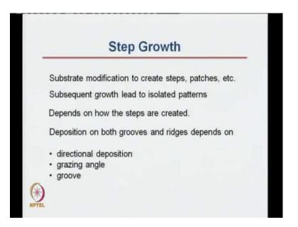
Subsequently, you can grow molecules to lead to isolated patterns. This will depend on of course, how you make the steps. So, the first step that you have to create steps or patches that will ultimately lead to the type of pattern you will get. So, it depends on how the steps are created then you can do deposition on both the grooves and the ridges that is between the steps. That depends on how you bring in your probe.
