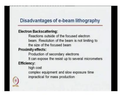
This e beam lithography can be used to develop specialized devices and prototype devices. The disadvantages of e beam lithography. There are couple of disadvantages for example, when you use an electron beam, there can be electrons which are backscattered like in an SEM you can always have electrons which are backscattered. Those electrons can give rise to reactions, which are outside of the focused electron beam.
