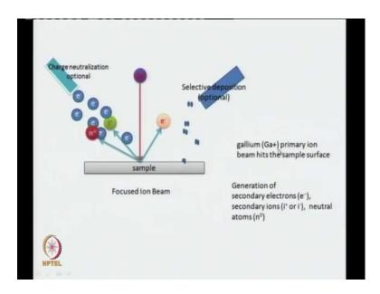
So, gallium ion is the primary ion beam which hits the sample. In this focused ion beam case you can have this beam falling on the sample and creating what are called secondary electrons. Then these secondary electrons can be used you can neutralize them if you want or you can additionally deposit something else, that is called selective deposition which is an optional aspect of this focused ion beam technique.
