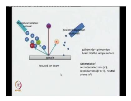
A schematic diagram of what happens in a typical focused ion beam. So, you have here you can what we generated here is the electron beam, but you can also have particles like gallium ions.
