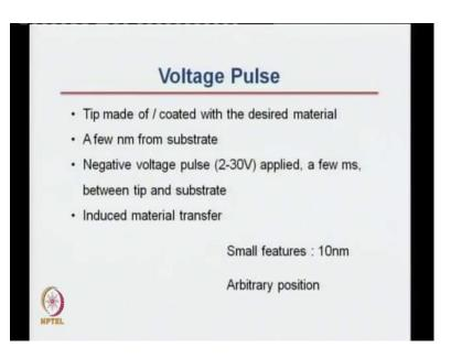
So, what is the voltage pulse technique. In the voltage pulse technique you make your coat the desired material which you want to pattern on a tip right. It can be made of the tip or it can be coated on the tip and it has to be brought close to the substrate. So, a few nanometers from the substrate. Then you apply a negative voltage pulse, say of the order of 2 to 30 volts and for a small time of few milliseconds between the tip and the substrate.
