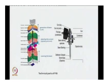
Now, if you that is a schematic diagram if you want to look at this focused ion beam equipment, the cross section or if a view inside it has got many parts. So, at the top in this focused ion beam system, you must have a source for ions because that is going to be the source for if you are going to use gallium ions, this is going to produce gallium ions. So, that is your ion source.
