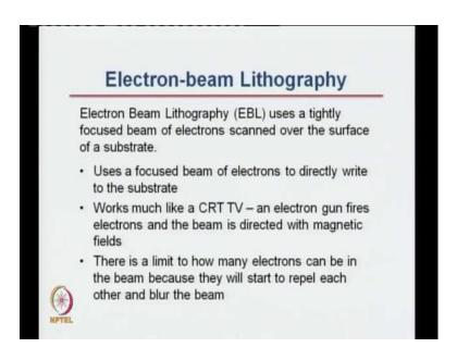
That will be used to make patterns on a substrate. So, this beam works very much the electron beam can be thought of which ordinary cathode ray tube, but which will be focused on a point using electromagnetic fields. There is a the number density of electron, that is how many electrons can be in the beam, there is a limitation because if you have too many number of electrons because electrons as you know are same charge, they have a negative charge they will start to repel each other.
