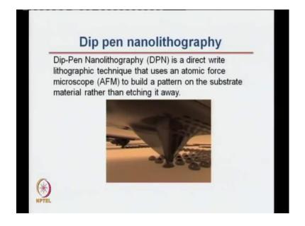
Now, move to another technique, which is a low cost technique, which is called dip pen nanolithography. So, if you go by the term dip pen, it is like you are having a pen and you are dipping it in an ink to write. So, it is this term dip pen nanolithography has emerged from that idea, that you have a probe which dips into a solution which contains some molecules, which you want to pattern on another surface.
