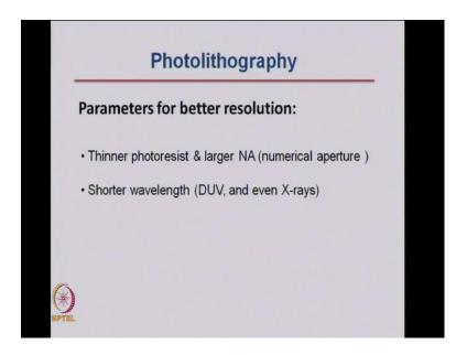
One thing is, which I already said that you need, for better resolution in photolithography, you need a large numerical aperture and short wavelength. In short wavelength you can go to deep UV extreme UV or even X-rays.
