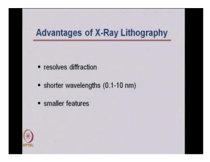
In photolithography, using UV, when we come across the problems of the diffraction limit, then if you use the X-ray techniques, which resolves that diffraction limit. Because, you can go to shorter and shorter wavelength like 0.1 to 10 nanometers and hence, you
