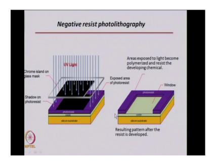
If you look at the negative resist photolithography, there it is just the opposite. It involves a photo resist, where if light falls on that photo resist that polymerizes. That will remain as such, it will polymerize. Wherever, light is not there, that can be moved. So, areas expose to light become polymerized and then when you add the whole thing to a developing chemical, the region where light was not falling, that does not resist the chemical and so, it will get dissolve.
