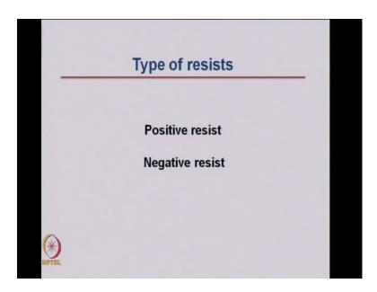
The types of resist are positive resist and negative resist. As you said, SU8 is a negative photo resist, but you can have both positive and negative resist. What is this positive and negative resist?
