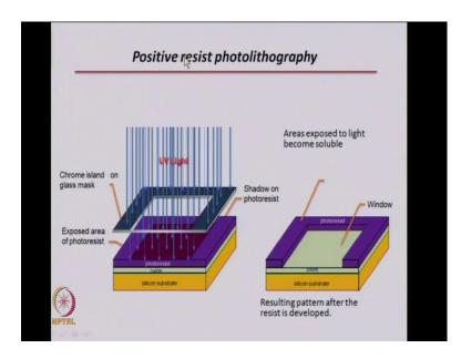
If you discuss this first, the positive resist photolithography, you have your substrate and then, this is your oxide layer; which is your film, in the previous slides we are talking of a film on a substrate. Here, that film is made of some oxide and then you have this photo resist on top of that, and then you have this mask. This mask can be some metal and which does not react, or is not sensitive to UV light.
