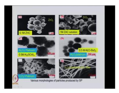
Very high there and you can see the type of a morphology is very different here. You have got spherical kind of structures, here you have a very irregular structures. So, the concentration and the type of agent that you are using is also different and that affects the morphology of these particles which you can see of the order of a micron or more.
