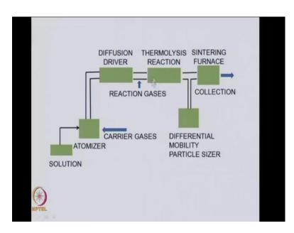
So, that is the overall mechanism how you go from the initial droplets used in spray pyrolysis when the droplets has generated by the atomizer to the final particle which is being deposited on the substrate.
