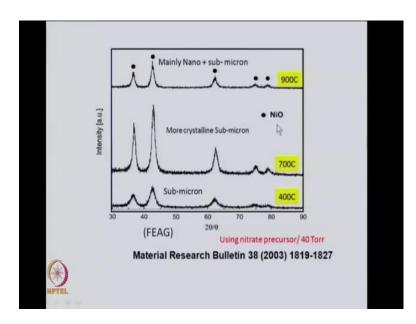
Whereas, at lower temperature you get the sub micron which particle, which are normally formed in any spray pyrolysis method. Then when you heat at 700 these sub micron particles crystallites, but when you are doing reaction at 900 then because the temperature is high.
