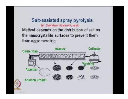
Then another method is the salt assisted spray pyrolysis this method is very simple. The same atomizer is there and carrier gas is there and you come to the furnace which is the
