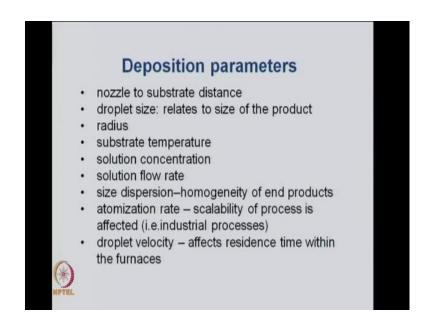
The initial precursor solution has a concentration and you can vary the concentration. So, that again is a parameter which can be varied. The solution flow rate can be varied that means the solution is coming into the atomizer at a certain flow rate say. So, many mile
