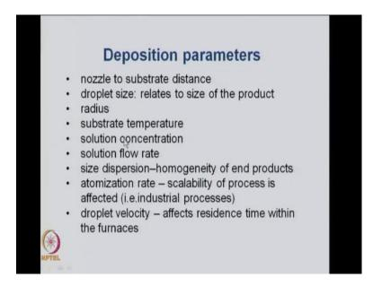
So, all this parameters will affect the size dispersion. That will affect the homogeneity of the final product which you get on the substrate. The atomization rate is very important because if you can do a very fast atomization.
