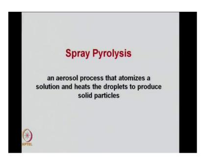
These spray pyrolysis method where which is very important from industrial point of view. Since, it is a simple method it is a scalable method can be applied to large areas and hence you can make lot of materials using this spray pyrolysis technique. From the words spray and pyrolysis you can understand that something will come out as an aerosol and will then be heated to produce the solid particles. So, pyrolysis is the term
