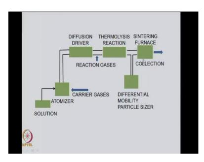
So, here you will keep your substrate they if the particles get sintered and the substrate will be at temperature which is set by this furnace. So, what is the substrate temperature is important.
