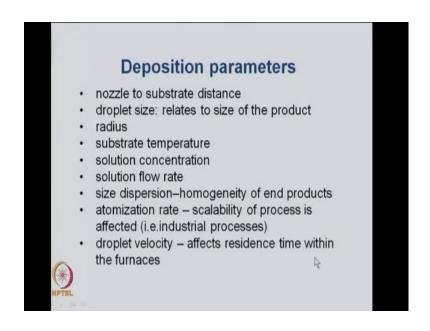
So, the droplet velocity will affect the residence time within the furnace and it will affect the size of the solute particles which will get deposited on the substrate. So, a large number of a parameters are there for 1 2 control and play with. So, that he can get precisely the type of sizes and size distribution of his particles as he wants. So, you have lot of room to play with, but also you need to have good control of these parameters otherwise the processes will not be reproducible.
