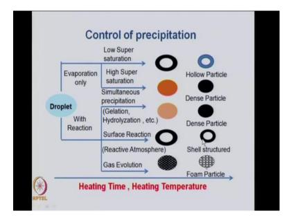
Can you introduce a reaction, and then you can get either dense particle or shell type of particle or a foam type of particle. So, by both these you can control the morphology or the nature of the particle from the droplet.
