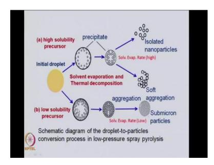
Now, depending on the starting precursor, you can have isolated nanoparticles or soft aggregation that means loosely held particles or very dense particles. That depends on the starting precursor. So, here if you have a very high solubility precursor, you see that you can initially the precipitate will have this kind of very fine particles which are separated well separated. So, you have an initial droplet which has very high solubility precursor that means solute is very well dispersed.
