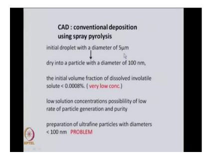
So, conventional deposition using spray pyrolysis has certain limitations because the initial droplet in a conventional spray pyrolysis has a diameter of around 5 micron. where has to make nanoparticles we need to have droplets a much smaller size.
