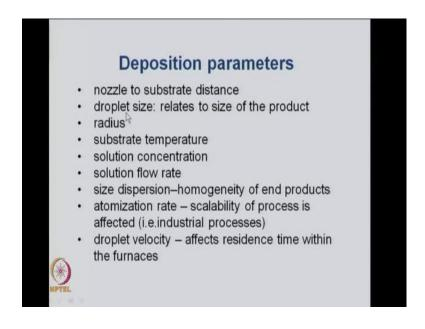
From there to the substrate there will be a certain distance. The droplets size how is the droplets size which is forming here. From here you are getting the droplets and forming here and going here to get the particles, how are these droplets size going to be varied depending on the atomizer, other parameters.
