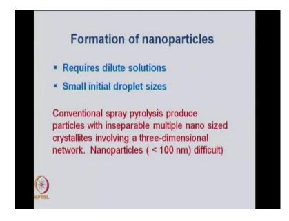
Now, these most of these conventional methods lead to formation of a submicron particles. As I said it may be 200 nanometers 300 nanometers 500 Nano maters etcetera, but if have to make nanoparticles less than 100 nanometers. So, 20 nanometers 50 nanometers using the spray pyrolysis method.
