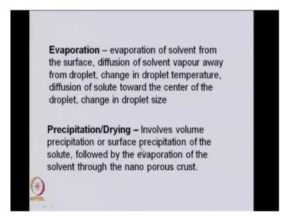
So, this mechanism of removal of solvent goes through these particular step. Through evaporation or precipitation drying ultimately leading to the submicron or nano particle.
