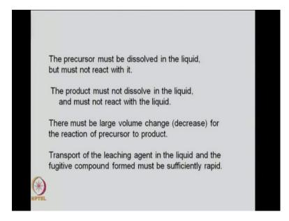
So, this is the solution based process of spray pyrolysis. In this spray pyrolysis method a certain factors need to be considered while during the process. The precursor that you choose must be dissolved in the liquid. Most of the time that is water and must not react
