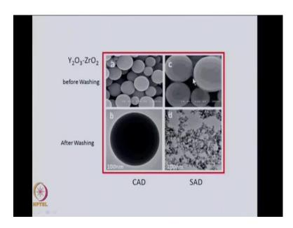
In the conventional method, this is the initial particle you get before washing. When you wash them you get these individual particles. In the salt assisted method; these are the initial particles that you get after washing you see you get very small particles, because all these particles now get a from here the salt gets removed and they break away into the small particles.
