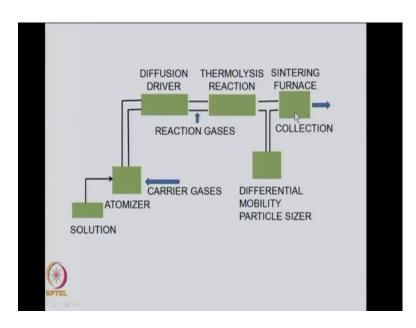
So, if you have these droplets which are coming here at low velocity then they will spend more time in the sintering furnace and the size will go up. However if the droplet velocity is very fast then the size will be small.
