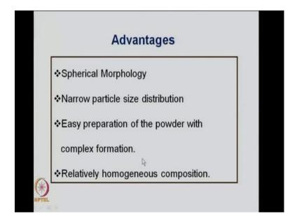
Now, the advantages are most to the time or most other spray pyrolysis processes. If you choose your starting precursors properly and choose you solvent also appropriately then you end of with particles with spherical morphology, with reasonably narrow particle size distribution. The process is quite simple and ultimately it is a good product for minimal investment. So, this has lot of advantages to take this process to the industrial scale.
