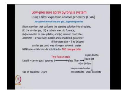
You are using there is abrupt evolution of heat and gas in this low pressure chamber, the particles becomes very small and you get this 20 nanometer particles.
