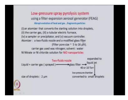
For example, you have the low pressure spray pyrolysis. In the low pressure spray pyrolysis system where there is a filter expansion aerosol generator, it is called FEAG. That allows an abrupt evolution of heat and gas and fragments the particles. So, this is a technique which has been develop is called the low pressure spray pyrolysis system with FEAG.
