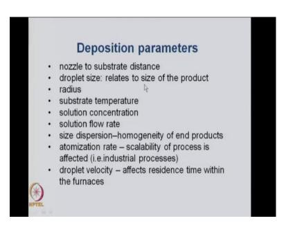
There is a relation if you change the droplet size, the particle size will change. Similarly, if you change the substrate temperature the particle size will change the substrate will be here we are trying to collect the sintered particles.
