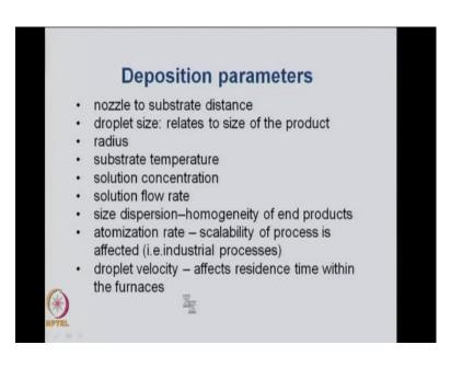
So, for industrial processes you need a very high atomization rate. So, the atomization rate needs to be scaled up for a processes which are going to be used in industry. The droplet velocity affects the residence time within the furnace.
