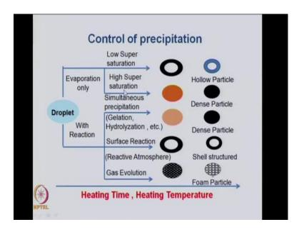
Of the starting materials because depends whether there is low super saturation that is high solubility or high super saturation that is low solubility. So, depends on the precipitation behavior by controlling the solubility or you can introduce a precipitation reaction into the droplet which is the second part.
