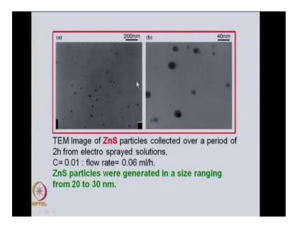
So, because of the electric field that you apply a cone is form and because of the cone the liquid comes out as a jet. This jet can be control to make particles of from 1 nanometer to several microns and these droplets when they are put on a substrate will gives you small particles like shown here.
