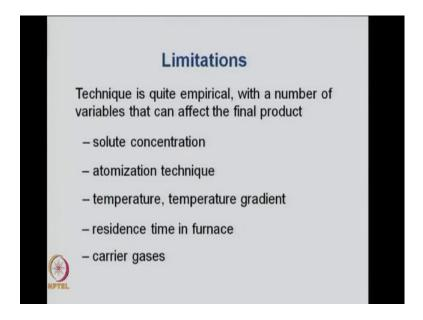
However, as with many most of the processes, there are certain limitations to this process too. The spray pyrolysis method is quite empirical with a large number or variables that can affect a final product. So, you have to optimize these parameters and hence when you move from one setup parameters to another setup parameters you might change the distribution of particle size in the final product, the size of the particles or the nature of the particles.
