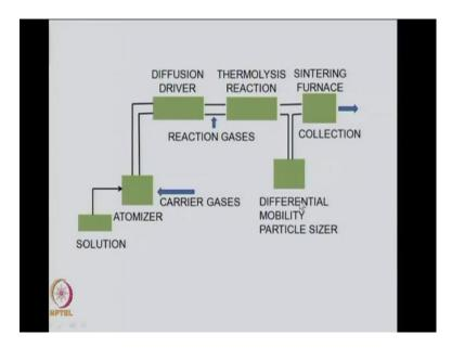
So, as we have to keep in mind not only the advantages of the method, but also the limitations of the method to make this technique a viable and useful for applications. So, this is a typical a semantic flow diagram of what happens in a spray pyrolysis method. So, here you have the solution where you have taken precursor and in a solvent and that goes to the atomizer.
