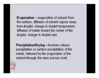
The solvent has to evaporates from the surface and the solvent has to diffuse the solvent vapour the gases that are forming due to the evaporation of the solvent have to move away from the droplet. This will cause a change in the droplet temperature and also diffusion of solute towards the center of the droplet. Ultimately this will bring about a change in the droplet size.
