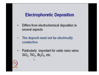
So far we discussed what is a electrochemical deposition and as we said, maybe repeatedly that electrochemical deposition is normally possible when you have a material which is highly conducting. So, what happens when you have materials which are not very conducting, for example like silica, or bismuth oxide or something like that. Then it is difficult to make wires out of them using the electrochemical technique. Then we use what is called the electrophoretic deposition technique.
