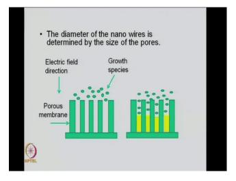
This is a clearer view of what one is doing. Here, you have the template as shown here. It can be like membranes, these are equally spaced templates and you want to grow your nanostructures within these cylindrical pores or cylindrical gaps and this diameter should be in the size of what you want. So, this should be if you want two nanometer or five nanometer wires then that should be the dimension of these cylindrical pores.
