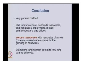
So, the conclusion is that this method is quite general. We can use this in fabrication of nanorods, nanowires and nanotubes of polymers, metals, semiconductors and oxides. You need to have porous membranes with nano size channels as templates and you can make wide variety of diameters, ranging from ten nanometer to hundred millimeter.
