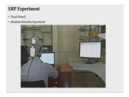
So, in the next video we will see one experiment you can see this is a setup for ERP experiment. So, here the subject is wearing an electrode cape and electrodes are here. This system which you can see here in which stimuli is being presented and here his potentials have been recorded.
