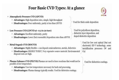
Now, in CVD we have seen four basic types of CVD. Like in PVD there are four categories in CVD also there are basic four categories. The first one you call is the atmospheric pressure CVD. And the advantages of it is high deposition rates, simple, high throughput, but the disadvantages are poor uniformity, purity is less than LPCVD. The low-pressure CVD is a second type of CVD in which we have the excellent uniformity and purity.
