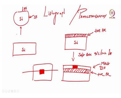
So, the next step is next step is, you soft bake it, soft bake at 90 degree for 1 minute on hot plate, after soft bake next step is you load the mask. So, I loaded the mask. What kind of mask? Bright field mask. This is again cross section of a mask, if I draw the top view this will look like this.
