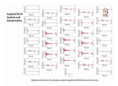
But when we go for an epilepsy by creating or by giving a drug to rats brain then you can see that there is seizure in several electrodes and here the value is 3000 micro volts. What was the value here? 200 microvolts which is normal ECOG signals versus 3000 microvolts because of the creation of the epilepsy and these are the seizures.
