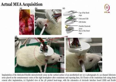
microelectrode array, and (d) and (e) The rat is immobilized in stereotaxic apparatus after implantation for in vivo experiments.
