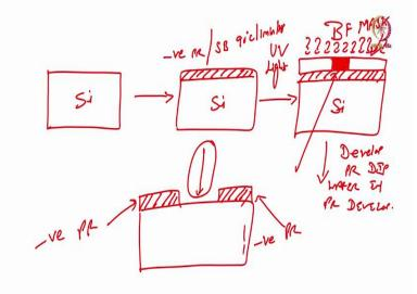
So, same process, I take a wafer, I coat the wafer with a photoresist, this time it is negative photoresist, next is I will spin, after coating the wafer, I will perform soft bake is the next 90 degree centigrade 1 minute hot plate. Next step is, load the mask. What kind of mask we have? We have a bright field mask.
