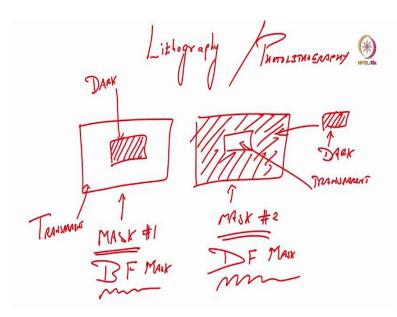
So, we are talking about lithography. And in lithography we are talking about photo lithography. So, lithography stands for carving from single stone, but here we are using photons which is light to create different structures. So, I will give you certain examples. So, let us start with two different examples, these are two different masks, what are these, mask.
