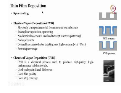
So, again there are two different things, one is a thin film deposition another one is thick film deposition. So, if you know screen printing, by which our greeting cards were initially produced, those screen technique techniques can be considered as a thick film technology. While thin film deposition, we have spin coaters, we have physical vapor deposition, we have chemical vapor deposition.
