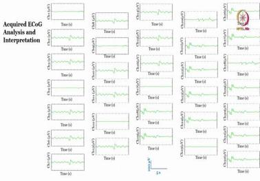
Baseline ECoG signals, after AED administration from all 32 channels, acquired using fabricated flexible microelectrode array,
