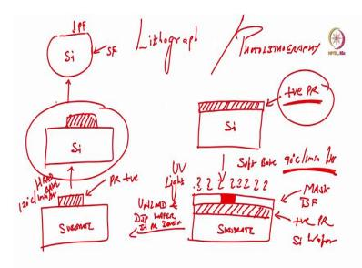
So, these are bright field mask. After bright field mask, next step is you expose this wafer to UV light. After exposing the wafer, you have to unload the wafer, unload the wafer and dip wafer unload the mask ok, unload the mask, do not unload the wafer. Then unload the mask and dip wafer is what the substrate right, generally we use silicon, so I say silicon wafer.
