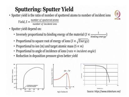
So, if you want to understand the yield of sputtering, then you need to understand how many number of sputter atoms versus how many number of incident ions. The higher the yield, that is S is higher; that means, better the sputtering efficiency, sputtering yield. Sputter yield depends on one inversely proportional to the binding energy of the material that is S is inversely proportional to the binding energy.
