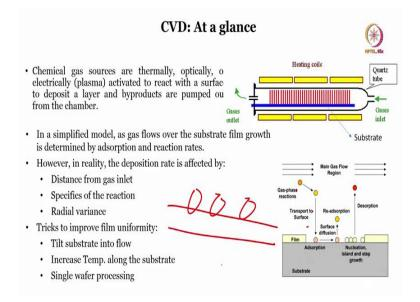
So, if you want to see the CVD at a glance then you know that there is a chamber, either this is vertical tube furnace, or it is a horizontal tube furnace in fact not vertical. Vertical tube furnace will come in this particular form, horizontal tube furnace is this one. So, this is a horizontal tube furnace and then, within that furnace we can load the wafers, these red lines are all wafers and then there are heating coils because you need to go for very high temperature.
