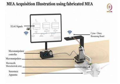
So, 1 shank versus 3 shank versus 4 shank versus 8 shank different electrodes are used for different regions. Here this particular region is hippocampus and then, if you want to acquire the signal, this is a schematic where you can load the micro electrode array onto the rat's brain.
