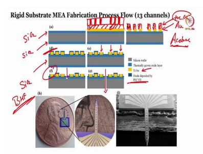
So, let us take an example of such a process and here is one of the processes so, what we have done is, you take a silicon wafer then you have an oxidized silicon which is blue
