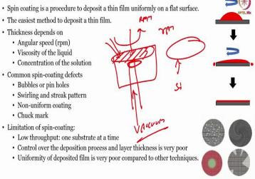
So, if you start with the spin coater spin coating is a procedure to deposit the thin film uniformly on a flat surface. Generally, we go for a photo resist coating. So, and there are several things that we need to understand, first is that this is the easiest method to deposit a film. So, what you do is, you take a spin coater, you load the wafer, there is a vacuum chuck which will hold the wafer and you spin this the wafer right at a given rotations per minute.
