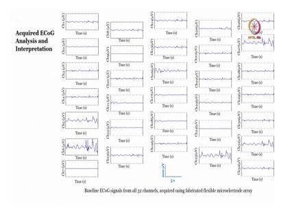
So, these are 32 signals acquired from all 32 electrodes, you have to see that the left side or the y axis is the voltage and x axis is time, time is in seconds and voltage is in micro volts you can see it is 200 microvolts and second is about 5 seconds.
