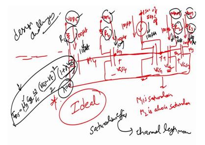
So, you have taken this transistor connected like this by pumping the current right you have generate you have generated the  $V_{GS1}$  that  $V_{GS1}$  you reflected on the another transistor ok that is nothing but  $V_{GS2}$  source are shorted and you have chosen R and D; R and  $V_{DD}$  in such a way that it is in also in saturation  $M_1$  is by default saturation  $M_2$  is also in saturation.
