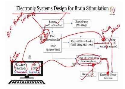
So, there is this switch, this is one of the requirements of our design. So, this is a switch here, you can program the switch from the microcontroller only if you close it, then you can go for stimulation if you open this then it is automatically into recording. So, what is this guy, open BCI Cyton-Daisy biosensing board, it will sense the potentials here and wirelessly transmits the signal to the GUI provided by the BCI.
