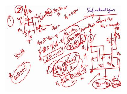
So, now, first you have to keep the transistor in saturation region. So, if you look at this guy. So, there is a point here, this point is nothing, but where your  $V_{DS} = V_{GS} - V_t$ , this is  $V_{DS} > V_{GS} - V_t$  and this is  $V_{DS} < V_{GS} - V_t$ .
