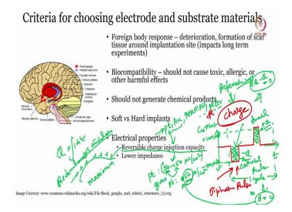
So, whenever you excite something, whenever you excite the membranes, brain membranes, when I say excite means you are inevitably charging, charge your transferring, through something like through capacitive means or faradaic means or both.
