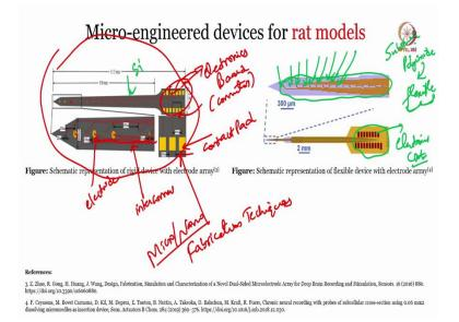
Now, you see this here, now let me erase this. So, this is electrode, and here it is a contact pad and these are interconnects, the red color things, these are interconnects which are connecting the electrode to the contact pad and here the electronics will sit.
