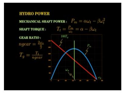
Now using that power equation the mechanical shaft power Pm which is equal to  $\alpha \omega t$ - $\beta \omega t^2$  see that torque and power are related torque into  $\omega$  is power so therefore torque the shaft torque can be obtained as power divided by  $\omega t$  angular velocity which is equal to  $\alpha$ - $\beta \omega t$  so this is the falling this is linear and falling slope now when t is 0 when the shaft torque is 0 you will see that  $\omega t$  is  $\alpha/\beta$ .
