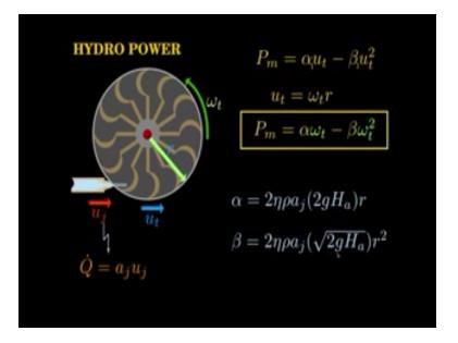
Now  $\mu t$  itself can be expressed in terms of the angular velocity so I have the radius r so  $\mu t$  is equal to  $\omega t^*r$  which is the radius of your inhaler now Pm can be expressed as  $\alpha \omega t$ - $\beta \omega t^2$  now this would be the power equation the mechanical power at available at the shaft there  $\alpha$  and  $\beta$  are given this one this can be as I said you substitute you will get this relationship.
