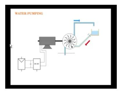
Another application of water pumping is in energy storage, recall in week 5 that we had discussed other forms of energy storage or pumped hydro was one of it. Here you lift water from the lower level to a higher level and store the energy in the form of potential energy, they lifted up potential energy of the water. And when you need it, you would like to convert that potential energy into kinetic energy may be simple as rotate.
