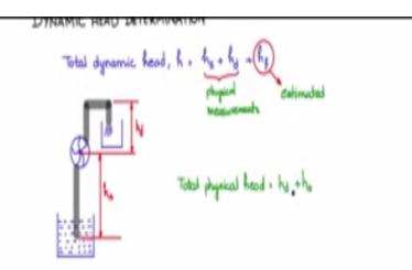
However for the case of pump if there is a sum which is down below the ground for the case of bore well where the water source is below the ground this is the total head that will come into picture the delivery head + the suction head and the delivery head will always add up.
