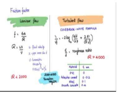
The friction factor is depended on the type of fluid flow see the fluid is incompressible most of the time what we are talking about is water pumping and therefore it is incompressible it is flowing through a pipe that are cylindrical the diameter is fixed therefore we can consider these two types we can consider these two types of flow that is the laminar flow, and the turbulent flow so the Reynolds number will indicate whether the laminar or turbulent, so let us say if the flow of a laminar.
