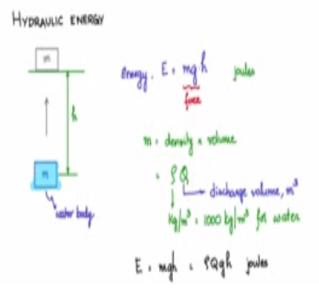
Let us now discuss the hydraulic energy that is required for lifting water from a lower level to a higher level that is for pumping water. Now let us say we have a mass which weighs M, M kgs and you want to lift it to a height H, so we want to bring this mass to this place which is at a height H from the original location.
