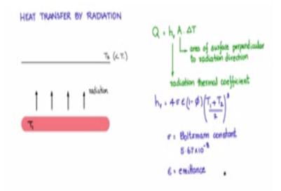
We had discussed heat transfer mechanism by conduction, heat transfer mechanism by convection free and forced convection. The third method, third mechanism for heat transfer is by radiation, radiation is a transfer mechanism from a hot body through electromagnetic waves, it does not need a medium for transferring the heat. So let us say that you have a hot body like this at temperature T1 and it is radiating heat through electromagnetic radiation.
