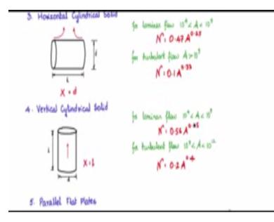
Recall that for the vertical cylinder laminar flow and the rally number is between  $10^4$  and  $10^9$  we use the Nussle's number relationship here which is given that  $0.56A^{0.25}$  so that is what we will be using.
