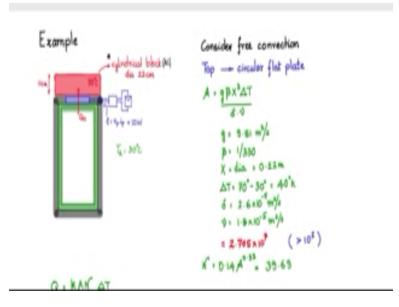
So recall this figure Qc is going to the cylindrical aluminum block is being transferred by the peltier junction there is amount of E electrical power which also goes in Qh here will be Qc+ E so Qc+ E amount is put into the external ambient and that is 24.39 watts.
