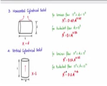
Is something like this we had discussed about the vertical cylindrical solid and the heat flow when it is placed in this fashion and we know that the characteristic dimension is l which is the height of the cylinder and for laminar flow and the turbulent flow the relationship for the Nussle's number with respect to the rally number is given in this fashion.
