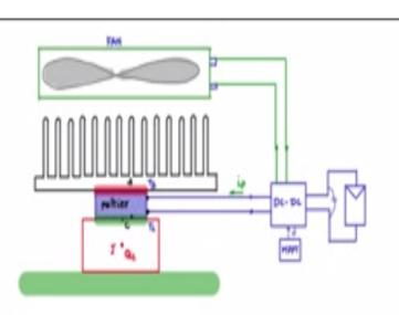
When you consider a peltier cooling system the peltier element itself is only one part of it. You see here that there is already a system which is generating heat and you want to cool it, you want to remove the heat that is dissipated, or this system, you have this red box here could be a box, the insights of which you would like to cool like in refrigeration.
