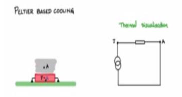
Let us discuss some examples on applications of peltier based cooling consider a PCB this green strip that you see here consider that it is a PCB on the top of that let us have a component which is becoming hot which is dissipating power so let me draw a component mounted on the PCB which is which dissipates power and it is our objective to remove the heat from it and then keep it within a rated temperature junction temperature such that it operates properly.
