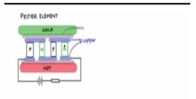
When the pass apply switched on V by this resistance plus the overall resistance between the terminal of the element will dictate the current flow and the current in this fashion it will take the path through this copper n block through this copper b block then n block b block so on.
