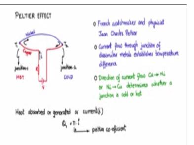
Consider two dissimilar metals, let us say one of the metal is nickel like this, it could be iron constant and nickel copper, copper aluminum. So there are many metal pairs that can be used. So let us say nickel and copper we use, this red line is the copper wire, blue line is the nickel wire. And let me connect it to a resistor and a potential source a battery like this.
