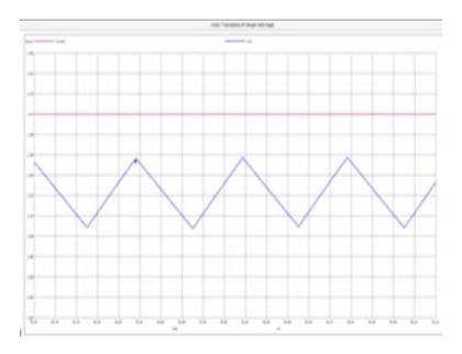
So the red one is iLref3 which is at 3 amps and let me expand it so and the blue is the inductor current, now you see that the inductor current is not reaching up to iLref the reason is that we have a slope compensated modified reference which is falling down from iLref value and when it is falling from iLref value the inductor current will cross it over somewhere less than IL rough value and change state and then start into the down slope mode.
